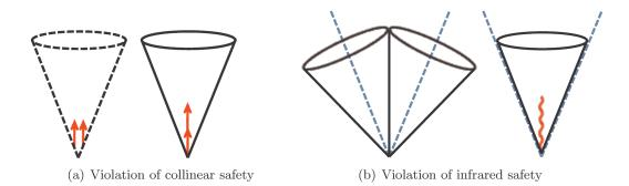
Figure 4.2.: Illustration of collinear and infrared safety: A collinear splitting should not lead to a difference in the number of reconstructed jets (a), nor should a soft emission (e.g. pile-up or underlying event) change the definition of the jet (b).
