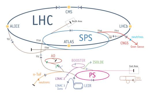
Figure 3.1.: The CERN accelerator complex, taken from [51]. Protons are pre-accelerated successively to higher energies in the Linac2, the Booster, the Proton Synchrotron (PS), the Super Proton Synchrotron (SPS) before injection into the Large Hadron Collider (LHC), where they are finally accelerated up to 7 TeV.
