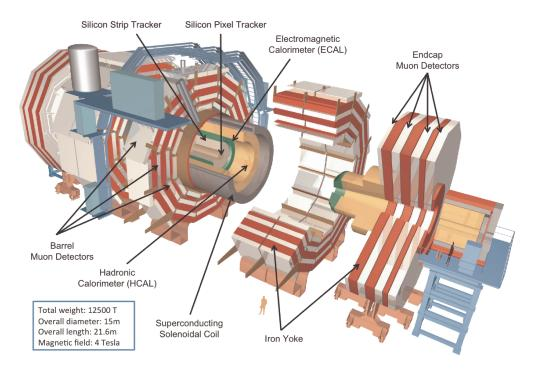
Figure 3.3.: Schematic overview of the Compact Muon Solenoid (CMS) detector, adapted from [62] with modifications. Note the symmetric and almost hermetic design around the beam pipe.
