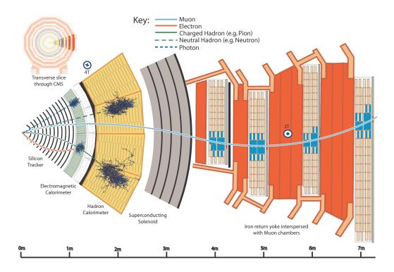
Figure 3.5.: Detection of particles in CMS [62], sketched in a transverse slice of the detector. Different particles are measured and identified by their characteristic behaviour under the influence of a magnetic field in the different sub-detectors.
