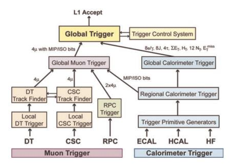
Figure 3.10.: Overview of the Level 1 Trigger architecture, taken from [63].
