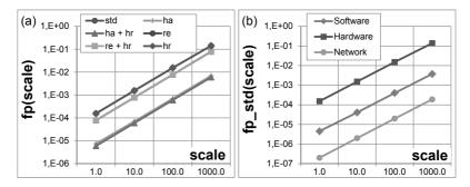
Figure 6.9: Audio Hosting Reliability Predictions with Varying Reliability Annotations, Based on the Single-Download Usage Scenario
