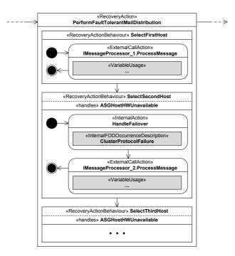
Figure 6.26: RDSEFF "ClusterProtocol.ProcessMessage" (Excerpt)
