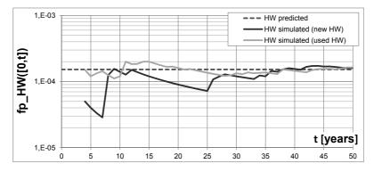
Figure 6.12: Variation of Hardware-Induced Reliability Impacts Depending on System Mission Time
