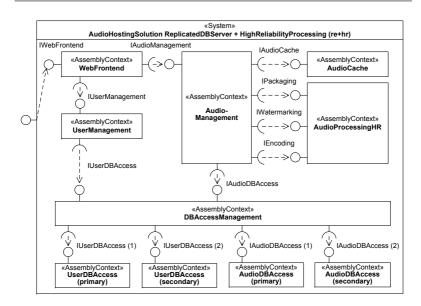
Figure 6.1: Audio Hosting System Model (re+hr)
