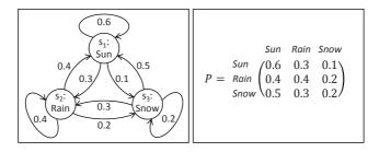
Figure 2.3: DTMC Example
