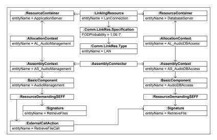
Figure 4.11: Network Reliability Specifications in the Audio Hosting Example
