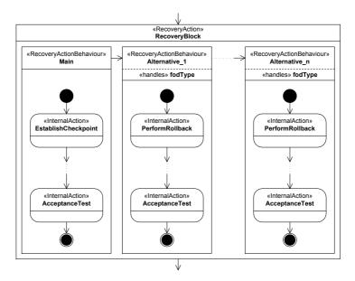
Figure 4.16: Recovery Block Example
