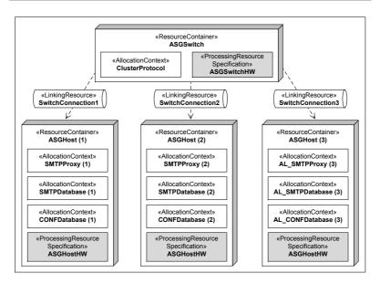
Figure 6.16: ASG Resource Environment and Allocation Model
