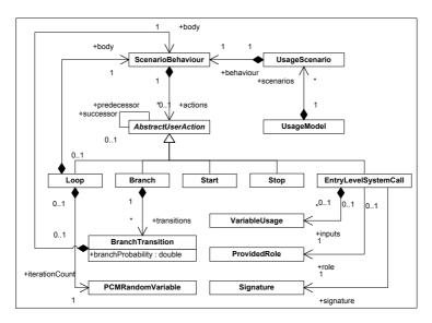
Figure 2.14: PCM Usage Meta-Model Classes
