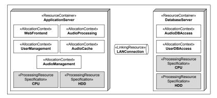
Figure 2.13: Audio Hosting Resource Environment and Allocation
