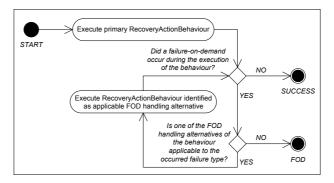
Figure 4.15: Execution Flow through Recovery Actions
