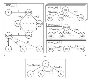
Figure 5.20: Evaluation of Remote Pointer Actions (Single-State)
