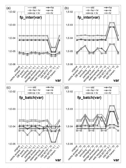
Figure 6.6: Robustness of Ranking of Design Alternatives Against Parameter Group Variations, Differentiated by Usage Scenarios and Change Directions
