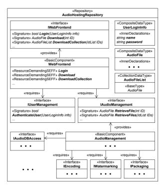
Figure 2.8: Repository Model for the Audio Hosting Example (Excerpt)
