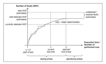
Figure 2.2: Software Reliability Growth Modelling Scheme
