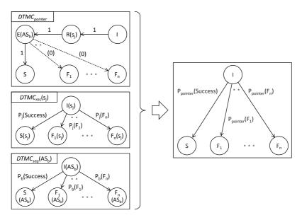
Figure 5.16: Evaluation of Entry-Level Pointer Actions
