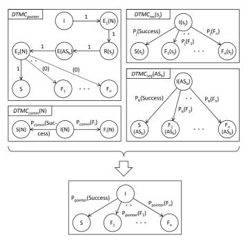
Figure 5.17: Evaluation of Remote Pointer Actions
