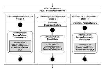
Figure 4.17: Multi-Stage Recovery Example
