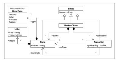
Figure 5.2: DTMC Meta-Model
