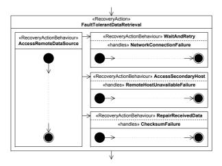
Figure 4.18: Multi-Type Recovery Example
