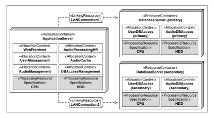
Figure 6.2: Audio Hosting Resource Environment and Allocation (re+hr)
