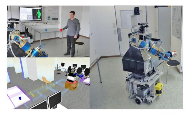
Figure 32: Pictures of exemplary PASE-3.1 situations: demonstration (top left), simulation (bottom left) and autonomous execution (right).
