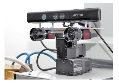
Figure 6: Camera head of Albert for machine vision with the Kinect camera on top and a Guppy Stereo-camera setup below.
