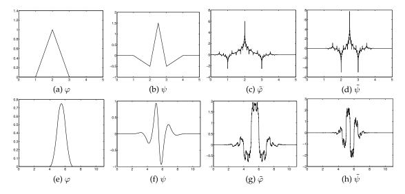
Figure 3.6.: *B-spline* scaling and wavelet functions on  $L_2(\mathbb{R})$  with m = 2,  $\tilde{m} = 2$  (top row) and m = 3,  $\tilde{m} = 5$  (bottom row).
