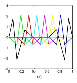
Figure 3.8.: Primal wavelet basis on the interval from [Pri09] with m = 2,  $\tilde{m} = 2$  and level j = 3.
