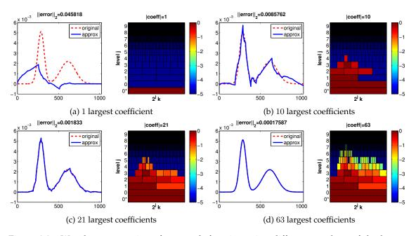
Figure 3.2.: Wavelet compression of a smooth function using different numbers of the largest wavelet coefficients. The approximation uses the *Daubechies db2* orthonormal wavelet basis. There are a total of 1024 coefficients in the wavelet expansion of the original function.
