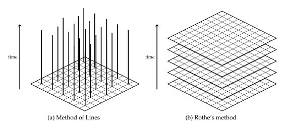
Figure 4.2.: Strategies for integrating the CME. In the left panel, the *method of lines* is shown (first space, then time discretization), while in the right panel *Rothe's method* is presented (first time, then space discretization) resulting in a series of stationary problems
