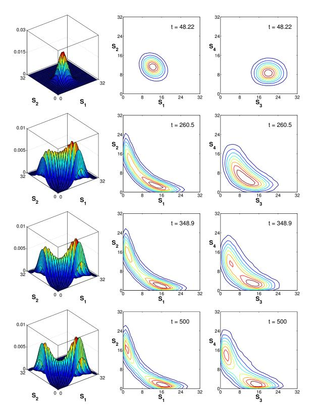
Figure 4.13.: Marginal distribution of the 4D toggle switch model (4.33) at different times. Surf plot (first column) and contour plots (second and third columns) of the approximation obtained with the adaptive wavelet method.
