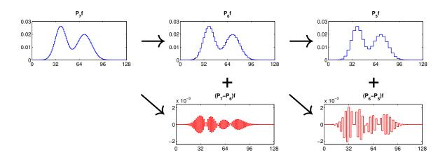
Figure 3.1.: Multi-scale decomposition via orthogonal projections using an orthonormal wavelet basis with m = 1 (Haar). The plots in the first row show successive approximations of the function f in increasingly coarser spaces  $S_j$ , while in the second row the details from the complement spaces  $W_j$  are shown.
