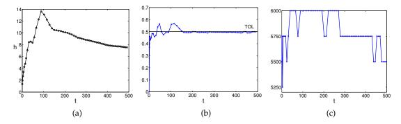
Figure 4.9.: Left panel (a): Evolution of step-size h for the 4D toggle switch. Middle panel (b): Evolution of the 1-norm (scaled) of the residual for the same problem. Right panel (c): Number of basis elements used in each step to compute the approximation.
