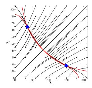
Figure 2.2.: Phase portrait of the deterministic reaction rate equations (2.96). Each black line represents a different trajectory of the deterministic process y(t) in the  $y_1y_2$ -plane. The initial conditions are represented by small black dots and the two steady states are depicted by blue circles. The null-clines  $(dy_1/dt = 0 \text{ and } dy_2/dt = 0)$  are depicted by red lines. Depending on the initial conditions, the deterministic process runs into one of the steady states.
