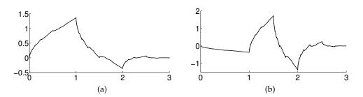
Figure 3.3.: Scaling function (3.3a) and mother wavelet (3.3b) of the *Daubechies db2* wavelet (m = 2)
