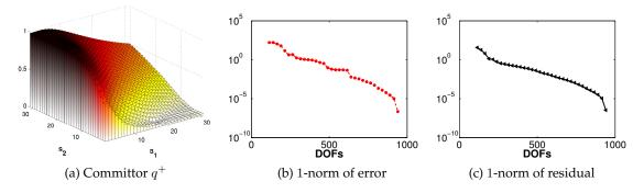
Figure 5.10.: Comparing the wavelet approximation of the forward committor function  $q^+$  for the model (2.94) with parameter set (4.32) with a reference solution obtained by solving the linear system (5.23) directly. Both the error and the residual of the wavelet approximation are measured in the 1-norm.
