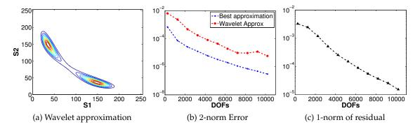
Figure 5.1.: Accuracy of the adaptive wavelet method for the stationary CME applied to the *toggle switch* model (2.94). Panel 5.1a shows a contour plot of the approximation obtained using the wavelet method with 3.5% of the total degrees of freedom, panel 5.1b compares the 2-norm errors of the truncated reference solution and that of the wavelet approximation, while in panel 5.1c we plot the evolution of the residual for the wavelet method.
