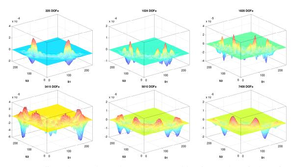
Figure 5.3.: Difference between the wavelet approximation and the reference solution for the *toggle switch* model (2.94), obtained with MATLAB's *eigs* command for increasingly refined active set of basis elements.
