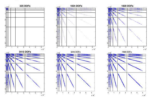
Figure 5.2.: Wavelet sets used by the adaptive wavelet method for the *toggle switch* model (2.94), plotted as sparsity pattern of the Petrov-Galerkin matrix for the full basis.
