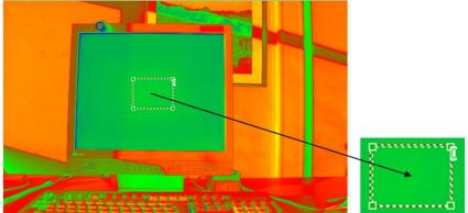
Figure 5–12: Luminance of the middle part of the monitor after and before reflection (in dark room and under daylight) are calculated to derive the reflection luminance on the exposed area during the reading test.
