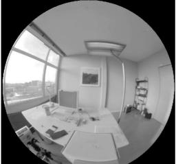
Figure 5–13: Fisheye pictures taken automatically every 30 seconds by means of a CCD camera close to subjects head position, these pictures are used to calculate the environmental luminance.
