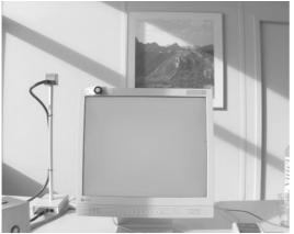
Figure 5–11: Monitor under daylight condition. As visible in this image the direct light from the outside is reflected on to the screen. Even such extreme cases are considered in the experiment to provide a dataset including all possible conditions for evaluation.
