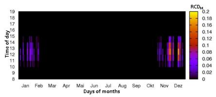
Figure 8–30: Annual veiling glare (RCD<sub>M</sub>) profile of variant 3-7: punched window façade without venetian blinds; screen position 7 (rated 17<sup>th</sup> from 24).
