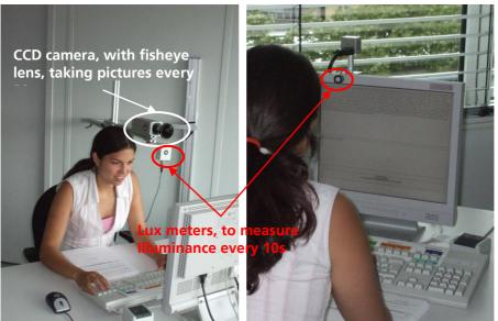
Figure 4–3: Images showing the test person by performing the test [54]. The CCD camera mounted on a tripod and positioned close to the subject's eye takes luminance pictures from the field of view every 30 seconds. The illuminance values close to the eye position and on the monitor corner and on the workplace are measured every 10 seconds using respective lux meters.
