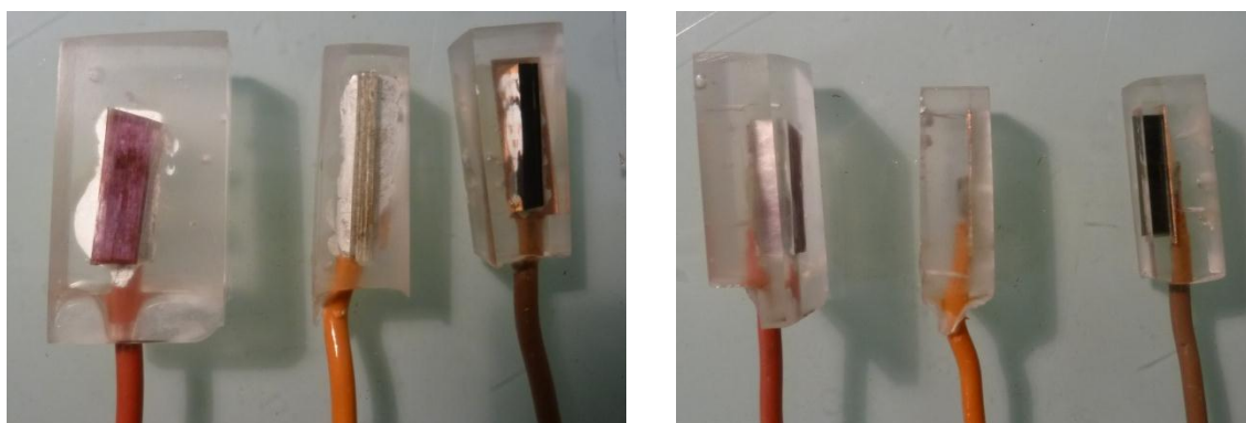
Figure 2: Views of three different electrodes. From left to right: lepidolite, muscovite and biotite.
