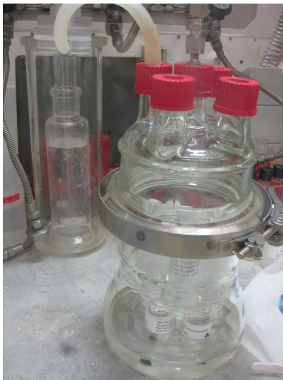
Figure 3: Start of the Pu(VI) reduction experiment. In foreground the reactor with five 20ml glass LSC vials (2x Fe coupon, 2x magnetite and one reference) and the oxygen trap in the middle of the reactor. In background the gas bubbling flask to determine the purging rate and act as water lock for oxygen intrusion.
