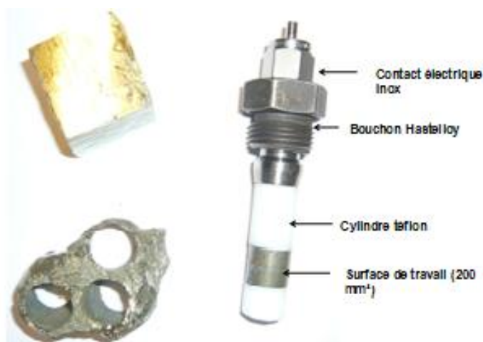
Figure 1: FeS_2 electrode made with "pure" Peruvian pyrite
