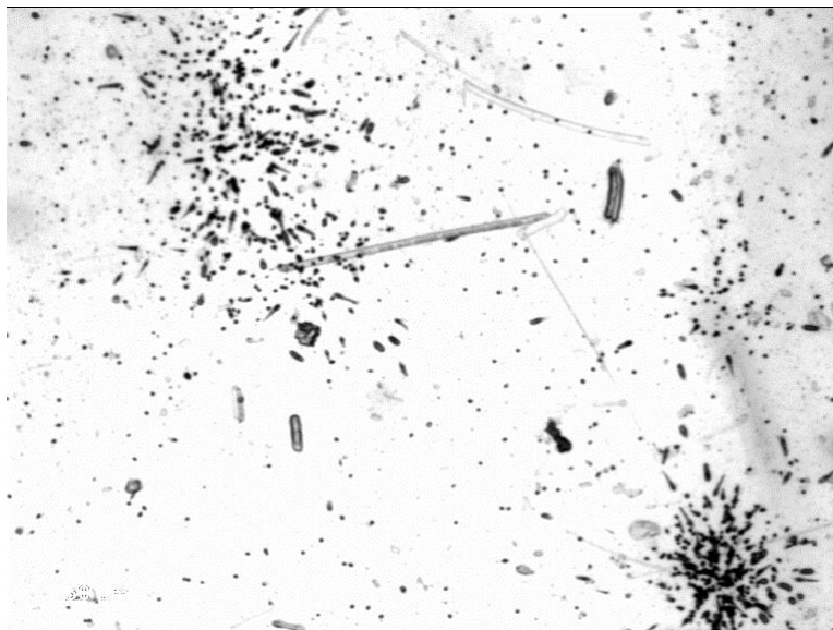
Figure 7: \alpha -tracks from Fe Magnetite 2 coupon (exposure time 1000 s, magnification 20x). The picture is a zoom-in on the upper left corner of Figure 6.
