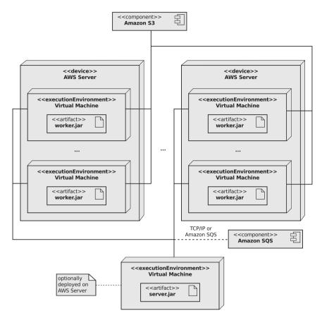
**Figure 6.9.:** UML deployment diagram for the MapPSO deployment in the Amazon Web Services<sup>TM</sup> (AWS) cloud infrastructure using the serverworker pattern.
