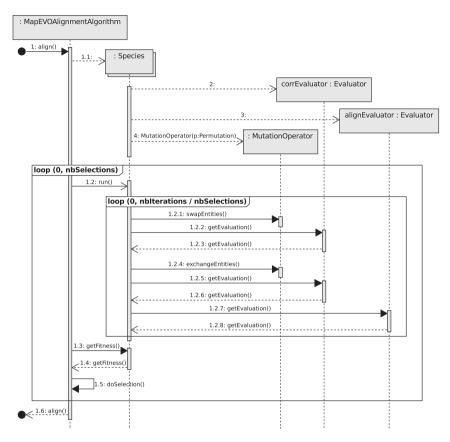
Figure 6.7.: UML sequence diagram of the MapEVO algorithm.
