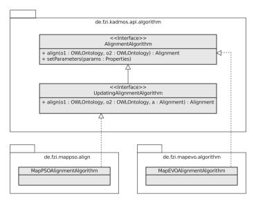
**Figure 6.6.:** UML class diagram for the MapEVO and MapPSO implementations of the *KADMOS* alignment algorithm interfaces.
