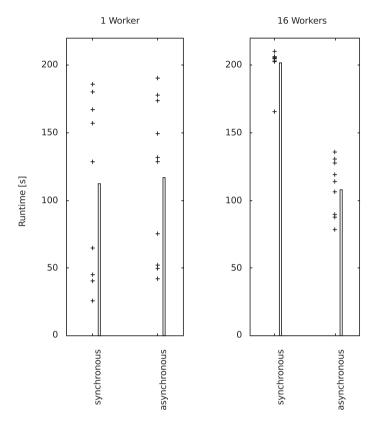
**Figure 6.10.:** Synchronous vs. asynchronous particle updates using 1 and 16 workers with 1 particle per worker. Bars denote an average of 10 runs (individual runs denoted left of the bars). Depicted is the total runtime for aligning the mouse ontology from the OAEI *anatomy* track (cf. Section 7.2.3) with itself.
