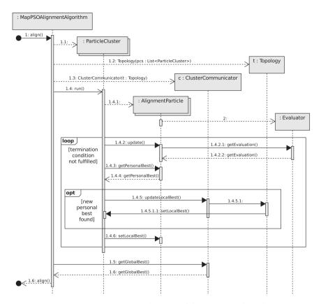
Figure 6.8.: UML sequence diagram of the MapPSO algorithm.
