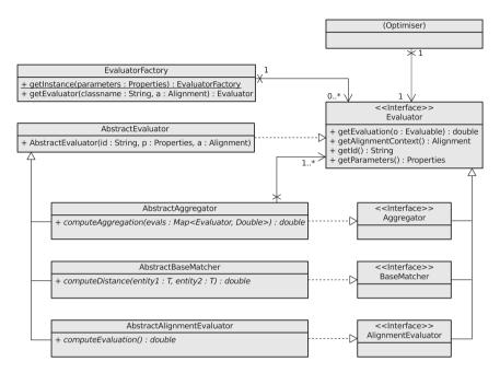
**Figure 6.3.:** UML class diagram of the *HARMONIA* Commons module for alignment evaluation.
