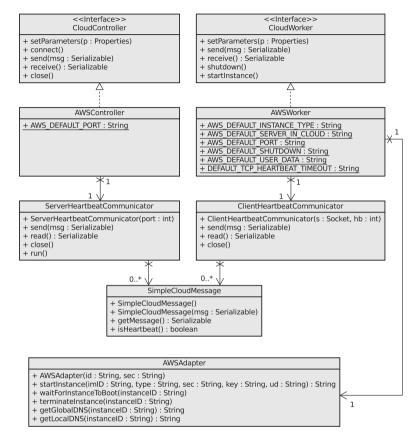
Figure 6.2.: UML class diagram of the KADMOS cloud adapter API.
