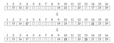
**Figure 5.7.:** Example application of the *swap* operator followed by the *exchange* operator on a correspondence permutation.
