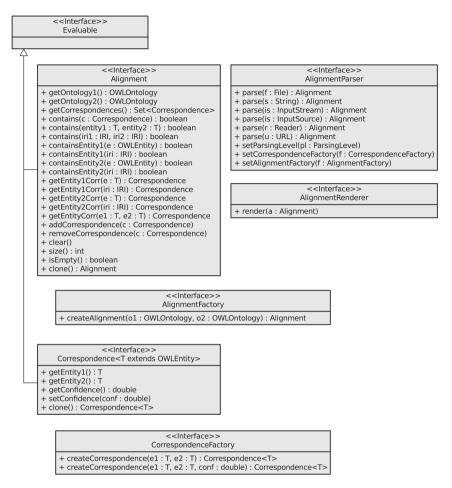
**Figure 6.1.:** UML class diagram of the *KADMOS* API.
