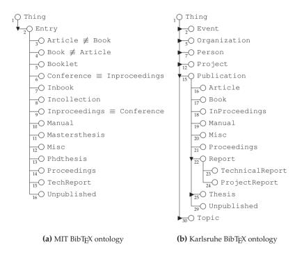
**Figure 1.1.:** Two example ontologies about the domain of bibliography. The figures show the class hierarchy of each ontology, which is only partially displayed/unfolded. Indented classes are subclasses of their parent, which denotes an *is-a* relationship between sub- and superclasses. Note that there is only a partial overlap between the two ontologies, since Ontology (b) covers a wider domain than Ontology (a).
