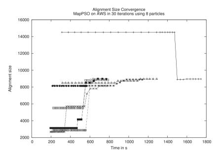
**Figure 7.11.:** Convergence behaviour of the MapPSO algorithm regarding alignment size on the AWS cloud infrastructure when aligning the Gene Ontology (GO) with the Medical Subject Headings (MeSH). Each line depicts the progress of a particle and line marks denote iterations.
