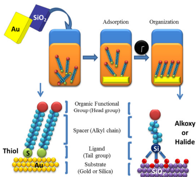
Figure 2.- Scheme of Self-assembled monolayers. The SAMs are commonly prepared by dipping the substrates in the solution containing the SAM molecule. The first step constitutes generally an adsorption onto the substrate followed by a reorganization of the alkyl chains. Generally the SAMs are created by two distinct molecules: thiols and silanes. The first uses a sulfur atom to bind onto gold and silver preferably. The second uses an alkoxy group to bind on oxidic surfaces such as silica or glass. They are constituted by three components: a) the organic functional group b) the spacer formed by an alkyl chain and c) ligand or tail group which binds to the substrate depending on the chemical group of the molecule.
