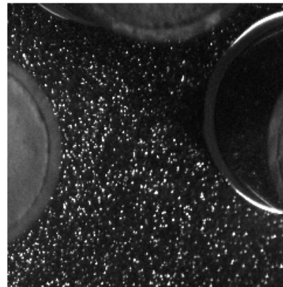
Figure 5 Example image for cross-correlation. Shown is a section of 238x244 pixel out of a 1600x1200 pixel image
