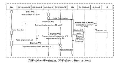
Figure 6.20: Workflow of the SPECjms2007 Interation 1 [Sachs 09]
