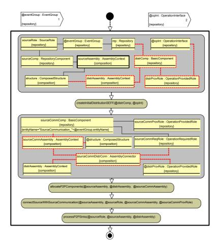
Figure 5.23: Sub-Procedure processP2PConnectors
