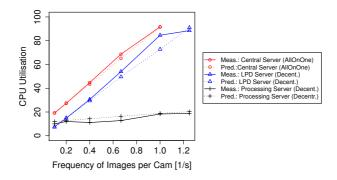
Figure 6.13: Scenario 2: Model Predictions Compared to Measurements
