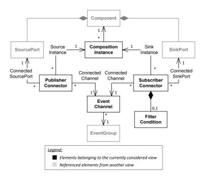
Figure 4.8: Modelling of Pub/Sub Connections
