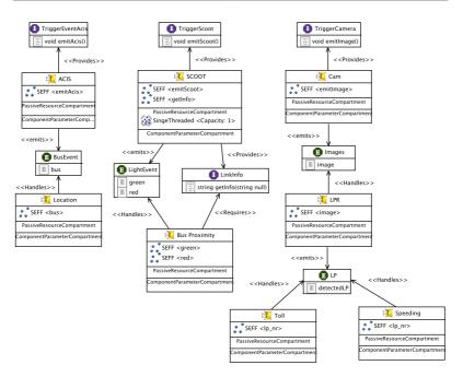
Figure 6.2: Component Repository of the Traffic Monitoring System
