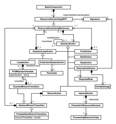
Figure 2.19: Meta Model of Resource Demanding Service Effect Specifications
