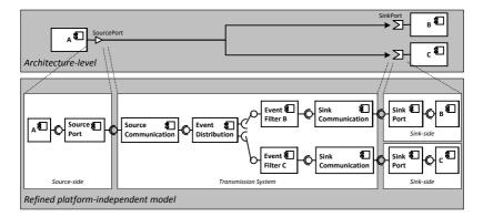
Figure 5.6: Refinement of a Source with Point-to-Point Connectors
