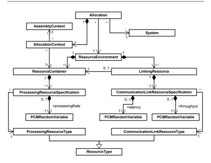
Figure 2.22: Meta Model of PCM Allocation Model and Resource Environment
