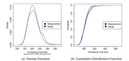
Figure 6.3: Measured and Predicted Processing Time Distribution
