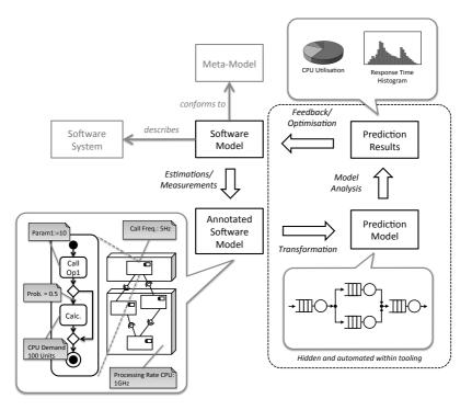
Figure 2.16: Model-based Prediction Process based on [Becker 08a]
