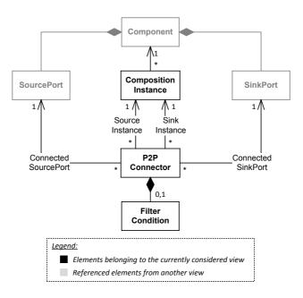
Figure 4.7: Modelling of P2P Connections
