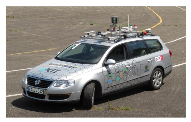
**Figure 1.1**: The experimental car *AnnieWAY* is equipped with numerous sensors and is capable of driving autonomously. The presented work focuses on data from the top mounted laser scanner and targets at sensing the environment.
