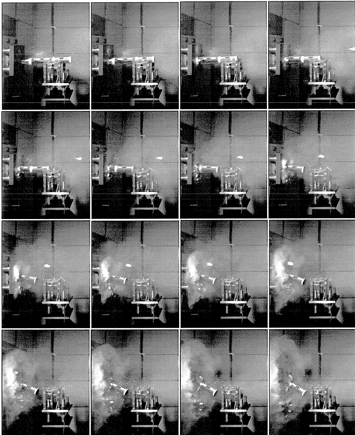
Figure 3 Picture sequence (frame rate 4000 frames/s) of a perpendicular impact ( \alpha = 0^\circ ) of a projectile with half-filled tank at a slow velocity
