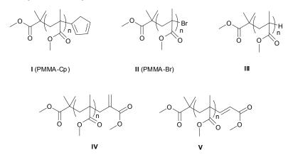
Scheme 4.2. Expected species during the ATRP process for the synthesis of PMMA-Br (II), and after elimination of Br (III), HBr (IV) and CH<sub>3</sub>Br (V).
