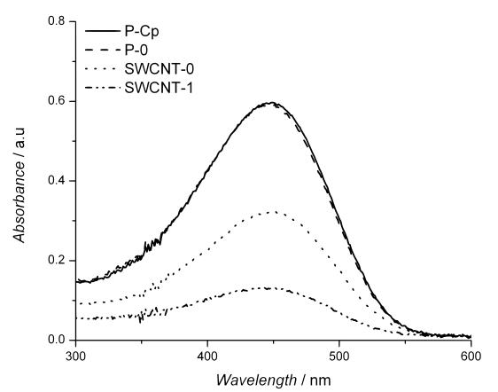
**Figure A13.** UV-VIS spectra of a 0.005 mM CHCl<sub>3</sub> solution of **P-Cp**, **P-0** and extracts from the dispersions prepared by 1 minute ultrasonication of 1 mg of **SWCNT-0** and **SWCNT-1** in 320 µL of CHCl<sub>3</sub>.
