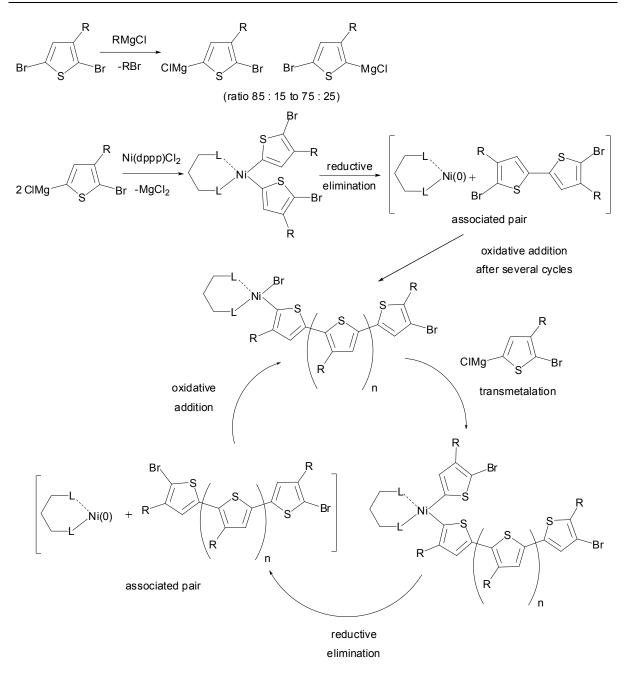
Scheme 2.6. Mechanism of GRIgnard Metathesis (GRIM) polymerization.
