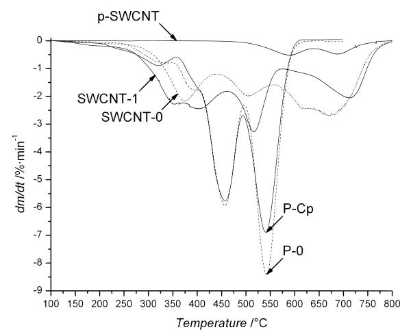
**Figure A11.** First derivatives of the thermogravimetric profiles of non-modified SWCNTs (**p-SWCNT**), cyclopentadienyl end-capped P3HT (**P-Cp**) and functionalized SWCNTs with **P-Cp** (**SWCNT-1**). The reference samples, non-functional P3HT (**P-0**) and the SWCNTs mixed with **P-0** (**SWCNT-0**) are represented. A heating rate of 10 °C·min<sup>-1</sup> was applied initially, following a 30 minutes isothermal step at 100 °C.
