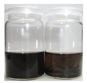
**Figure A14.** Digital photograph of the dispersions prepared after 1 minute ultrasonication of 1 mg of **SWCNT-1** (left) and **SWCNT-0** (right) in 10 mL of CHCl<sub>3</sub> after 5 days.
