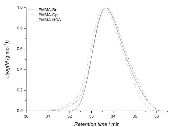
**Figure A15.** SEC traces of the starting material **PMMA-Br** ( $M_n = 2700 \text{ g} \cdot \text{mol}^{-1}$ , D = 1.14), the Cp-end capped **PMMA-Cp** ( $M_n = 2700 \text{ g} \cdot \text{mol}^{-1}$ , D = 1.17), and after the HDA reaction with **Dithio-OH** (**PMMA-HDA**,  $M_n = 2900 \text{ g} \cdot \text{mol}^{-1}$ , D = 1.16).
