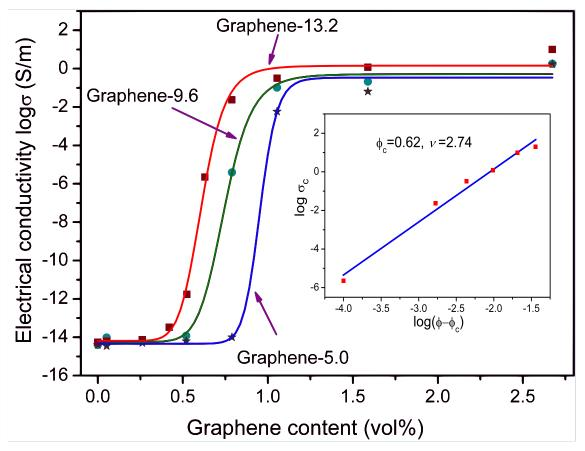
**Figure 2.3.** Electrical conductivity of graphene/PMMA composites as a function of graphene content characterized by different C/O ratios (5.0, 9.6 and 13.2 via XPS). Reproduced with permission from Ref. 126 (Zhang *et al.*). Copyright 2012, Elsevier.
