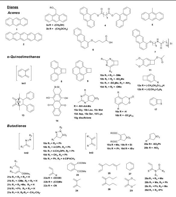
Scheme 2.1. Dienes (acenes, *o*-quinodimethanes, butadienes) reacting via DA reaction with carbon materials. The *o*-quinodimethane model intermediate (Int1) is generated by 8-17, and the butadiene model intermediates Int2 and Int3 from 18a-e and 19a-20b respectively. The yields and reaction parameters with specific carbon materials are collated in Table 2.1.
