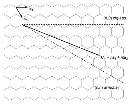
**Figure 2.1.** Representation of the graphene sheet and the chiral vector  $C_h$  of the SWCNTs.  $a_1$  and  $a_2$  are unit vectors (norm  $a_{C-C} \cdot \sqrt{3} = 2.46$  Å). The configuration (n, m) represents the armchair SWCNTs, (n, 0) the zig-zag SWCNTs, and any other (n, m) pairs chiral SWCNTs.
