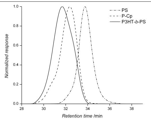
Figure 6.7. Overlay of SEC traces of P-Cp, RAFT synthesized PS with dithioester endgroups, and P3HT-*b*-PS synthesized via HDA ligation.
