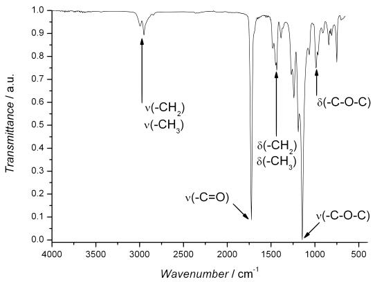
Figure A19. FTIR spectrum of PMMA-Cp in a KBr pellet.
