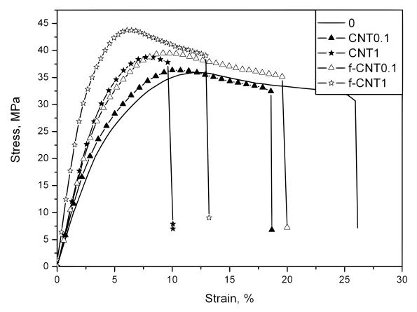
**Figure 2.4.** Stress-strain plots of isotactic poly(propylene) composites of 0.1 to 1.0 *wt.-%* of untreated and phenol functionalized MWCNTs. Reproduced with permission from Ref. 129 (Selvin *et al.*). Copyright 2012, Wiley-VCH.
