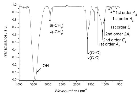
**Figure A18.** FTIR spectrum of the pristine SWCNTs (**p-SWCNT**) in a KBr pellet. The identified peaks agree well with those reported in the literature.<sup>353</sup>
