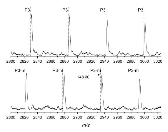
**Figure 5.7.** ESI-MS spectra of doubly charged PNIPAM with Cp end-group conjugated with *N*-maleimide (**P3-m**) in THF. All spectra are recorded via direct infusion.
