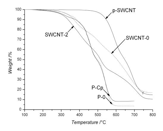
**Figure 6.8.** Thermogravimetric profiles of non-modified SWCNTs (**p-SWCNT**), cyclopentadienyl end-capped P3HT (**P-Cp**) and functionalized SWCNTs with **P-Cp** (**SWCNT-1**). Profiles of the non-functional P3HT (**P-0**) and the reference sample SWCNTs mixed with **P-0** (**SWCNT-0**) are also shown. A heating rate of 10 °C·min<sup>-1</sup> was applied, following a 30 minutes isothermal step at 100 °C.
