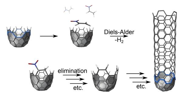
**Figure 2.2.** *Polymer approach'* for the synthesis of SWCNTs via successive DA reactions of nitroethylene on a CNT end cap and subsequent elimination reactions. Reproduced with permission from Ref.104 (Schrettl *et al*). Copyright 2012, Wiley-VCH.
