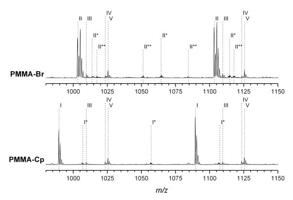
Figure 4.3. ESI-MS spectra of PMMA-Br (II) and PMMA-Cp (I) polymer obtained via direct source infusion. Signals marked with an asterisk represent double charged species (\*) and triple charged species (\*\*). Minor side products from ATRP process (III, IV, V) are also identified.
