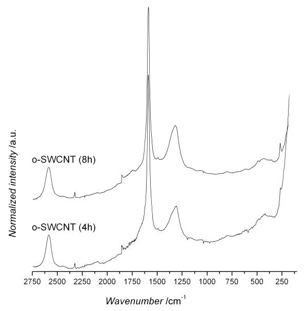
**Figure A17.** Raman spectra of oxidized **o-SWCNT** after 4 h and 8 h acidic treatment. The spectra were recorded in water dispersion with a 785 nm laser excitation after purification, and normalized to the G-band peak intensity.
