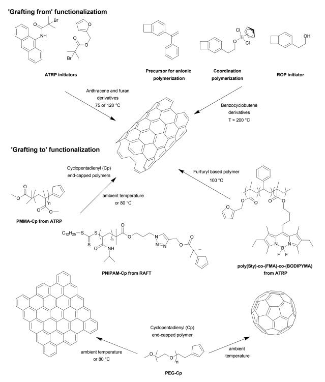
**Scheme 2.3.** Polymer functionalization of fullerenes, CNTs and graphene via DA reaction performed via *'grafting from'* and *'grafting to'* approaches. Five-membered ring functionalities react under mild conditions (ambient temperature to 80 °C).
