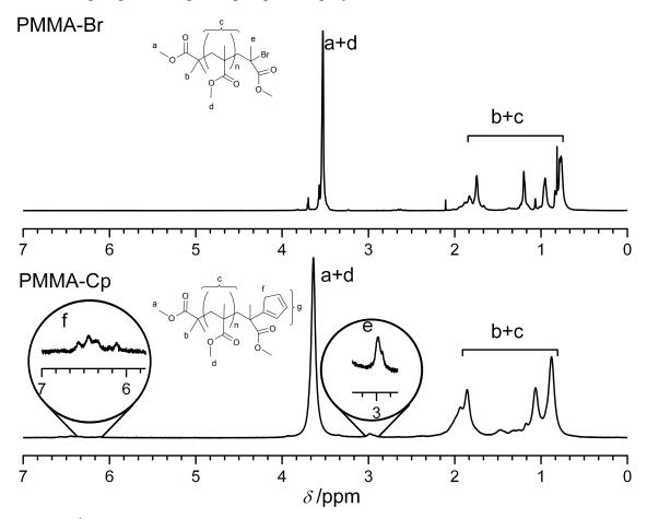
**Figure 4.2**. <sup>1</sup>H NMR spectra of the starting material PMMA-Br (top) and the final PMMA-Cp (bottom) after the end-group modification.
