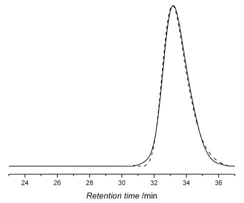
Figure 4.1. SEC traces of PMMA-Br (dot line) and PMMA-Cp (continuous line).
