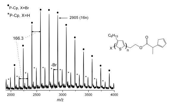
**Figure 6.3.** MALDI-ToF mass spectrum of **P-Cp**. The major peak series corresponds to **P-Cp** with X=Br while the minor peak series represents **P-Cp** with X=H. For both series the difference between two consecutive peaks matches the mass of P3HT repeat units. For a detailed peak assignment refer to **Table 6.1**.
