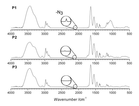
**Figure 5.4.** FTIR spectra of PNIPAM with different end-group (azide, **P1**), (bromine, **P2**), and (Cp, **P3**) in KBr pellets with recognizable azide peak for **P1** at 2096 cm<sup>-1</sup> (zoomed part of the spectra).
