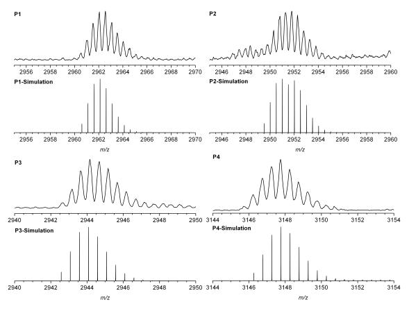
Figure 5.6. ESI-MS isotopic pattern of doubly charged PNIPAM with different end-groups (upper spectra) and the respective simulated isotopic pattern (lower spectra): P1 (azide, top left spectra), P2 (bromine, top right), P3 (Cp, bottom left) and P4 (acidic end-group, bottom right). The spectra are recorded via direct infusion.
