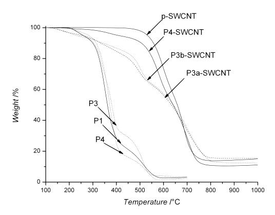
**Figure 5.8.** Thermogravimetric profiles of PNIPAM with different end-groups (azide, **P1**), (Cp, **P3**) and (acid, **P4**), as well as pristine SWCNTs (**p-SWCNT**), functionalized with Cp-terminated PNIPAM at ambient temperature (**P3a-SWCNT**), and at 80 °C (**P3b-SWCNT**). All samples are measured in air atmosphere with a heat flow of 10 °C·min<sup>-1</sup>, undergoing a preliminary isothermal step at 100 °C for 30 minutes.
