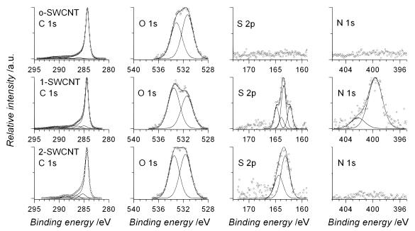
**Figure 7.5.** XPS spectra of SWCNTs after each functionalization step for each constituting atom (C, O, S and N): after oxidation (**o-SWCNT**, top), after esterification with **Dithio-OH** leading to **1-SWCNT** (middle), after HDA reaction with **PMMA-Cp** leading to **2-SWCNT** (bottom). For a better visualization, all spectra are normalized to maximal intensity.
