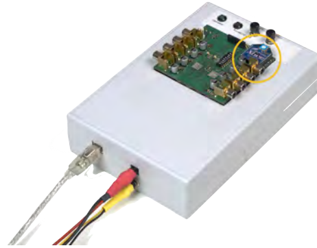
Fig. 6. Signal Generator Unit used for sound signal generation and amplification as well as radio pulse emission. The orange circle highlights the 2.4 GHz radio module.
