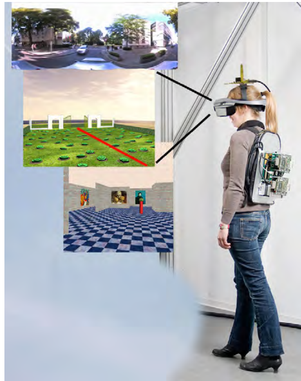
Fig. 1. User wearing the telepresence system. The depicted scenarios are (top to bottom): A spherical street panorama, a minesweeper game, and a virtual museum tour.
