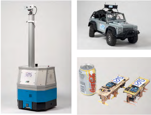
Fig. 2. Teleoperators involved in the telepresence environment at the ISAS laboratory. Left: The Omnibase [2], an omnidirectional robot platform with pan-tilt stereo cameras. Top right: Radio controlled, teleoperated off-road vehicle. Bottom right: 6DOF miniature walking robots.
