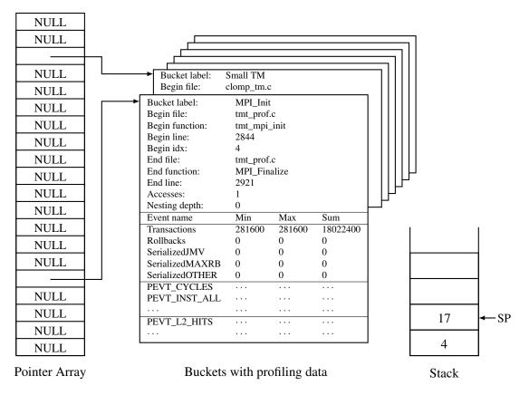
Figure 9.1: Data structures of the profiling tool for TM with a simplified example showing two nested buckets.
