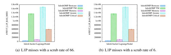
Figure 9.21: L1P misses with LULESH and 16 threads executed in long-running mode.
