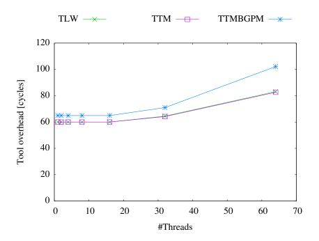
Figure 9.4: Tool overhead for measuring an empty code region with three different levels of information and over multiple thread counts for the TM overhead tool.
