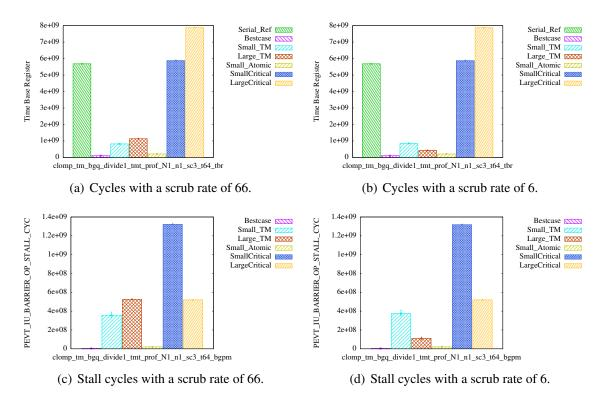
Figure 9.9: Stall cycles as an indicator for adjusting the scrub rate in the short-running mode. Run with clomp\_tm\_divide1 64 1 64 100 128 None 3 1 0 sr 100.
