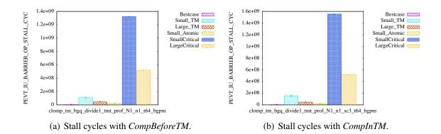
Figure 9.15: Studying the influence of setting the scrub rate on the stall cycles with the long-running mode. Run with clomp\_tm\_divide1 64 1 64 100 128 None 3 1 0 6 100.
