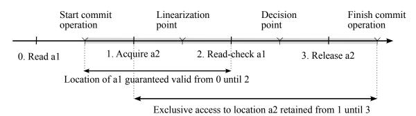
Figure 2.1: Illustration of commit phases in a Software Transactional Memory system; taken from Fraser and Harris [67].
