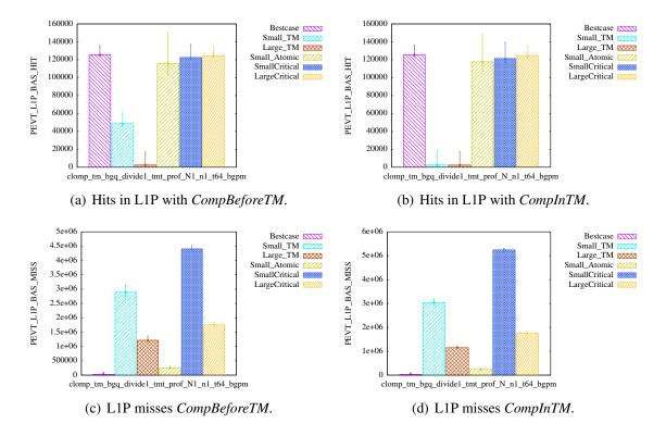
Figure 9.14: Studying the influence of moving the computation inside the transaction in the long-running mode. Run with clomp\_tm\_divide1 -1 1 64 100 128 None 3 1 0 6 100.
