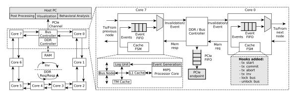
Figure 5.9: An 8-core TMbox system block diagram and modifications made to enable logging of events (shown in gray) – taken from [189].
