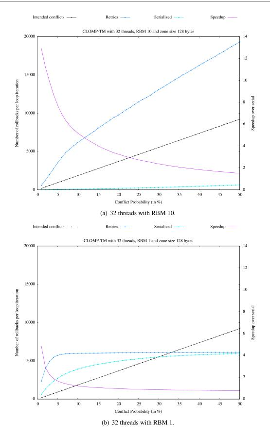
Figure 8.5: Influence of TM\_MAX\_NUM\_ROLLBACK (RBM) on retries/speedup. Run with clomp-tm-bgq-divide1 -1 1 x1 d6144 128 firstZone, cp, randFirstZone 3 1 0 6 100. First published in [171].
