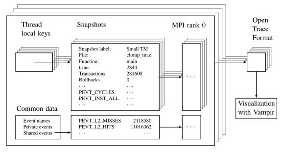
Figure 9.2: Overview of the tracing tool for TM with data structures and work flow.
