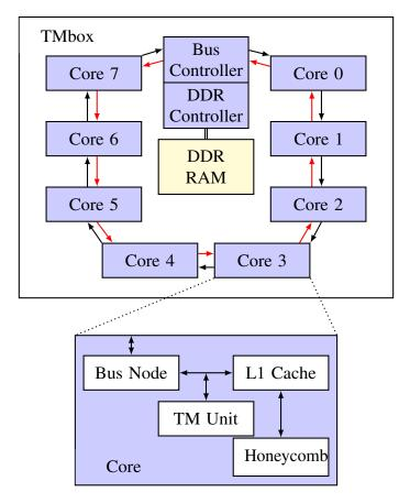
Figure 5.8: Overview of the TMbox system, showing a bi-directonial ring bus that connects 8 cores and a bus controller (similar to [190]).
