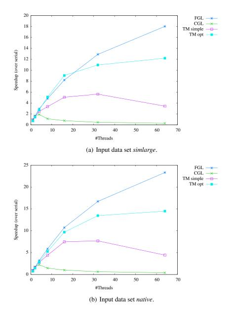
Figure 8.10: fluidanimate with coarse-grained and fine-grained locking as well as simple and optimized transactions.
