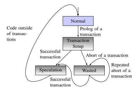
Figure 9.3: Finite state machine that describes how the transactional actions select the correct bucket.
