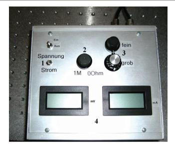
Fig. 7.10.: Battery-driven source developed to bias the YBCO detectors. (1) Switch to change between voltage and current biasing. (2) Knob to enable a short-cut of the detector bias line. (3) Coarse and fine regulator to adjust the bias current/voltage. (4) Displays showing the bias current and voltage of the detector.
