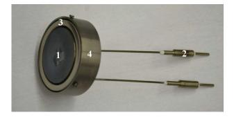
Fig. 4.6.: Oxygen-compatible heater with stainless steel heating plate (1) with embedded heater spiral with cold ends (2), a ceramic shield (3) and an outer stainless steel shielding (4).
