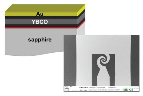
Fig. 2.4.: Multilayer structure and final layout of the new YBCO THz direct detector technology.
