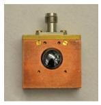
Fig. 7.2.: The YBCO detector block made from copper for good thermal contact to the cold plate. The detector chip is glued to the embedded silicon lens and rearside-illuminated [TSH<sup>+</sup>12].
