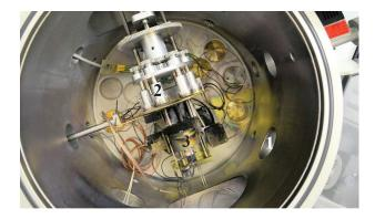
Fig. 4.5.: Inside of the deposition chamber: The laser beam enters the chamber through the window (1) and hits the target at the target carousel (2). The ablated material is deposited onto the substrates situated on the heater (3).
