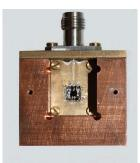
Fig. 7.3.: The YBCO detector chip mounted to the rear-side of the silicon lens is connected via indium bonds to the Rogers substrate.
