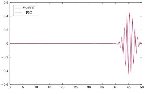
Figure 7.17: Comparison of YeeFCT and PIC for  $E_y$  at  $t/T_0 \approx 50$
