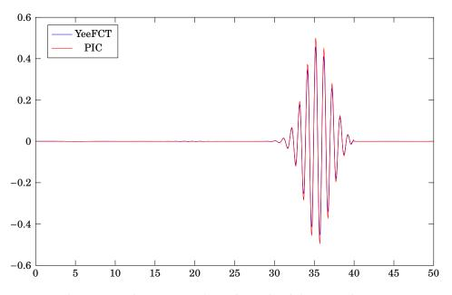
Figure 7.15: Comparison of YeeFCT and PIC for  $B_z$  at  $t/T_0 \approx 40$
