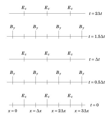
Figure 2.2: Space-time chart of the Yee algorithm for a one-dimensional example
