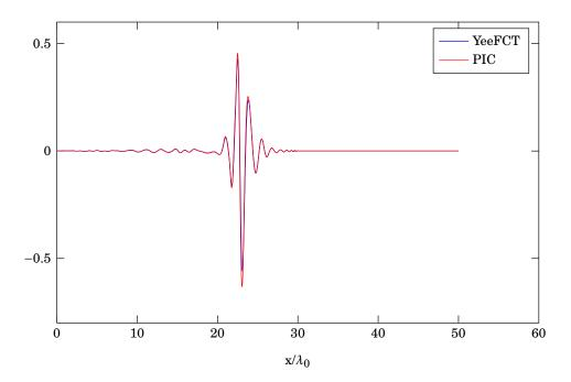
Figure 7.28: Comparison of YeeFCT and PIC for  $B_z$  at  $t/T_0 \approx 30$
