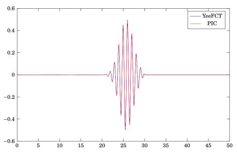
Figure 7.12: Comparison of YeeFCT and PIC for  $B_z$  at  $t/T_0 \approx 30$
