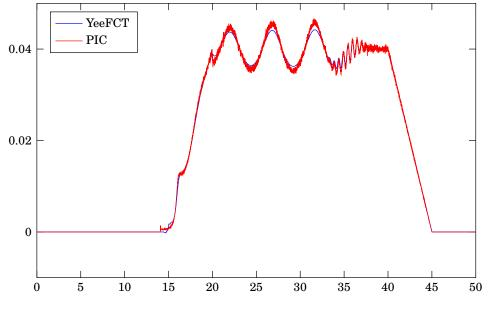
Figure 7.13: Comparison of YeeFCT and PIC at  $t/T_0 \approx 40$
