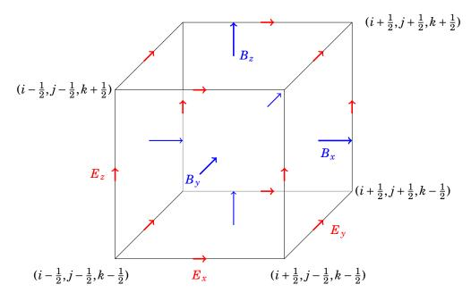
Figure 2.1: Schematic view of a 3D Yee cell
