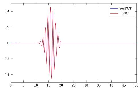
*Figure 7.9:* Comparison of YeeFCT and PIC for  $B_z$  at  $t/T_0 \approx 20$
