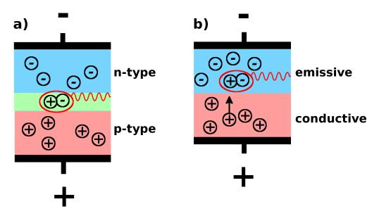
**Fig. 7.1.:** Differences between semiconductor LED and organic LED. a) A pn-junction of a semiconductor LED. When applying a voltage, holes and electrons travel to the junction between the p- and n-doped semiconductors. They recombine emitting a photon. b) Holes inside the conductive layer diffuse into the emissive layer. Electrons and holes recombine in the emissive layer and emit a photon.
