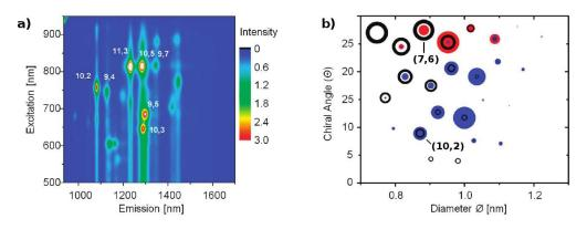
**Fig. 7.10.:** Fractions of nanotube content observed using Photoluminescence Excitation. a) PLE image of nanotubes dispersed with polymer 1 in toluene. b) Merged intensities transformed into the diameter/chiral angle plane. Blue: PLE signal observed in solution dispersed by polymer 1, Red: PLE signal observed in solution dispersed by Na-cholate in  $D_2$  O. Images courtesy of Lemasson et. al[283].
