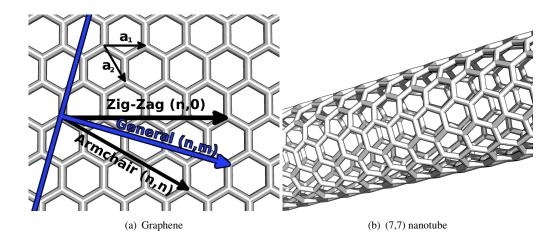
**Fig. 7.6.:** Graphene sheet and carbon nanotube. a) A flat graphene sheet.  $a_1$  and  $a_2$  are the lattice vectors of the unit cell. A nanotube is defined solely by its chiral indices (n, m). The tube is rolled along the blue axis orthogonal to the lattice vector. Two specific nanotube configurations are drawn: an armchair tube (n,n) and a zig-zag tube (n,0) b) A rolled up (7,7) armchair nanotube for comparison.
