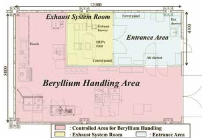
Fig.3 Partitions in the Beryllium Handling Room.
