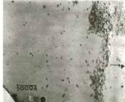
Fig. 2. Electron micrograph showing loops on {1120} planes in quenched and annealed hot pressed beryllium.
