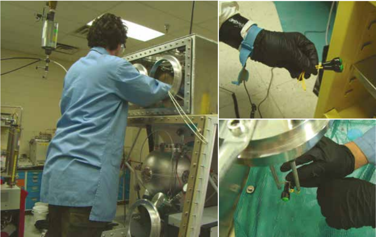
Fig. 2-3. Wiring igniters in ExCEED.
