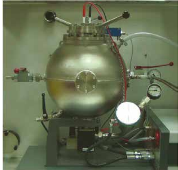
Fig. 2-1. Schematic [7] and photo of the Kühner 20 liter sphere in ExCEED. The vacuum ball valve and vacuum gauge, not shown in the schematic, are visible at the right in the photo.
