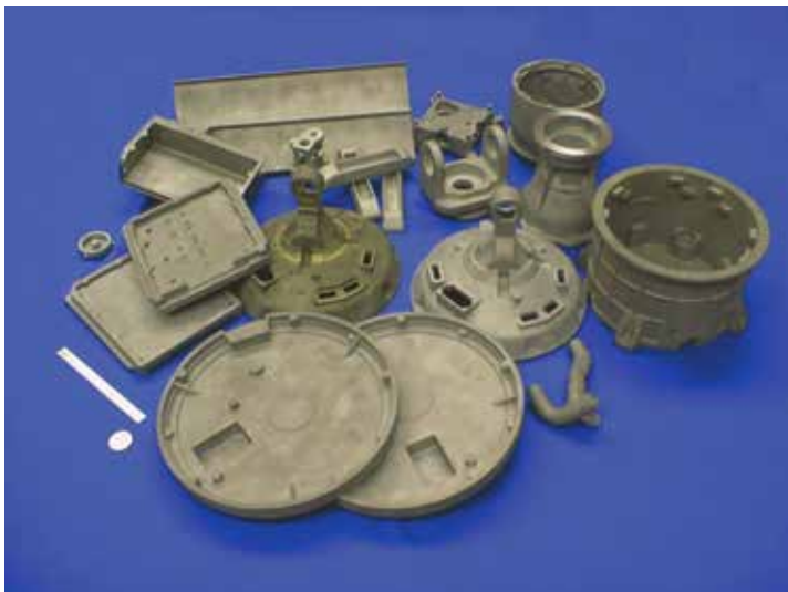
Figure 6 —A variety of components that have been investment cast at Materion using AlBeCast® 910.
