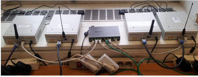
Fig. 6: The test setup for the first live testing, using four USRP N210
