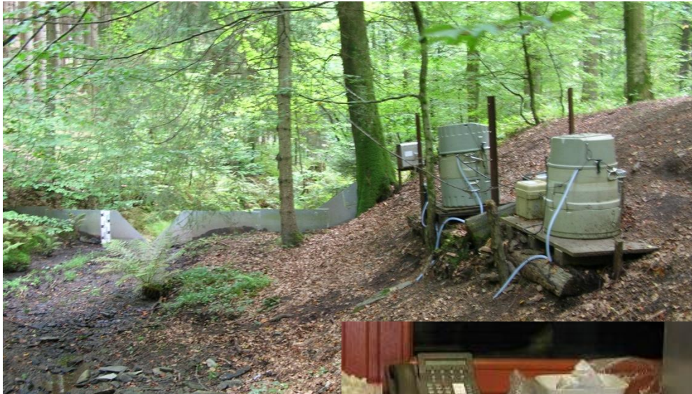
Automatic water sampling Weierbach, Luxembourg (A. Krein, CRP-GL)
