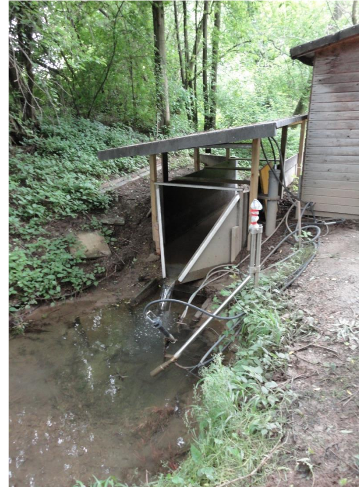
Turbidity probe in the HOAL catchment, Petzenkirchen, Austria
