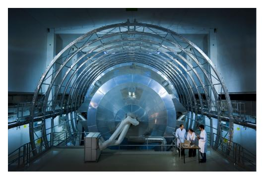
Figure 2.7: Photograph of the main spectrometer, surrounded by the large volume air coil system (photo: KIT).
