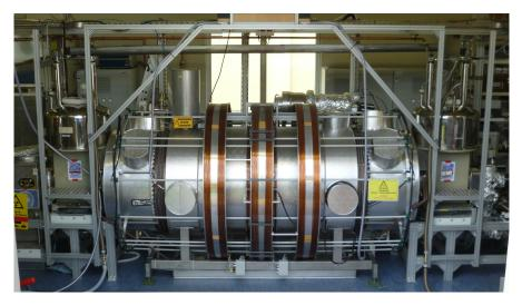
**Figure 2.8:** Monitor spectrometer, installed at the KIT site. Two solenoids and 4 air coils (3 visible, 4<sup>th</sup> hidden by the middle one) produce the magnetic guiding field.
