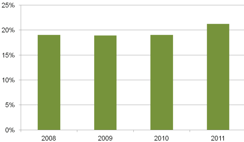
Figure 2.1.: Total electricity exports and imports as shares in total electricity generation in the EU-27 and Norway.
