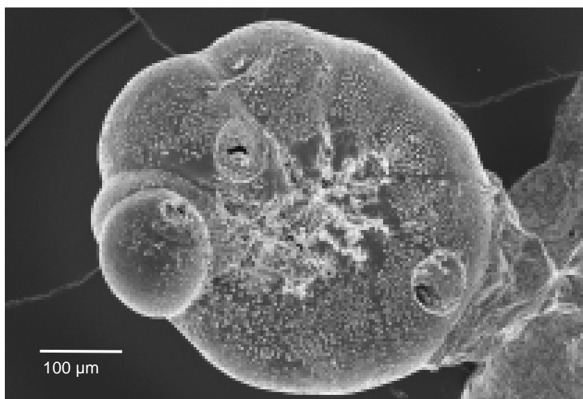
Figure 32 – SEM micrograph of a foraminifer with ablation craters showing balloon-like newly formed chamber in the front
