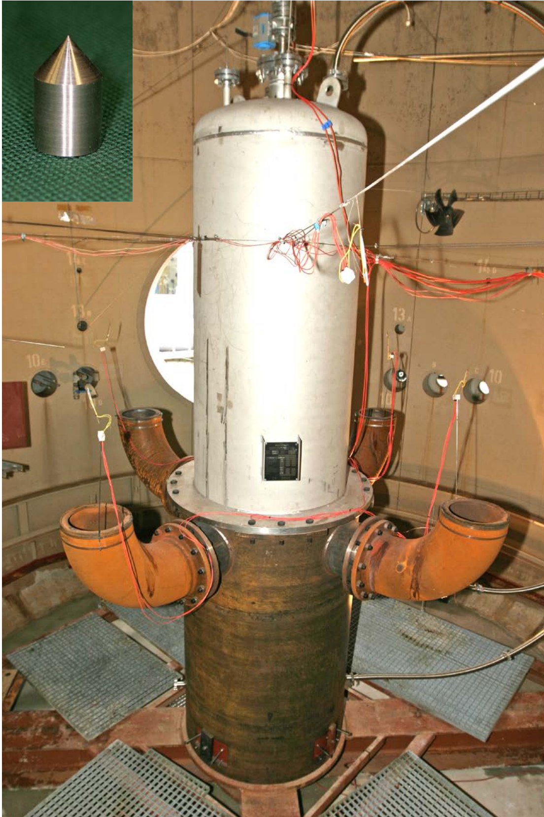
Fig. 6. Inside pressure containment vessel with RPV/RCS-vessel and cavity; plunger
