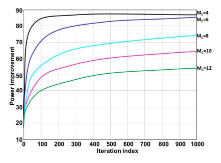
Figure 4.8: Illustration of the OBCL synchronization efficiency for different values of M
