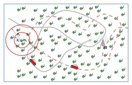
Figure 1.3: Illustration of the positive effects of CC on the network connectivity of MWSNs
