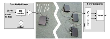
(a) Test scenario: relation of the USRPs (center), transmitter block diagram (left) and receiver block diagram (right)
