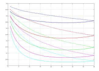
Figure 3.12: Comparison of the minimum number of C-nodes to gain different levels of BER for the proposed and conventional methods
