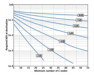
Figure 3.8: Impact of the number of C-nodes on BER (Labels of the curves represent the average SNR at C-nodes)
