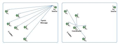
(a) C-nodes receive the signal of the source (b) C-nodes interact to the destination for synchronization
