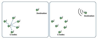
(a) Full-feedback Closed-loop phase syn- (b) Open-loop compensation of the phase chronization (interactions are among C- errors due to different position of the C-nodes) nodes
