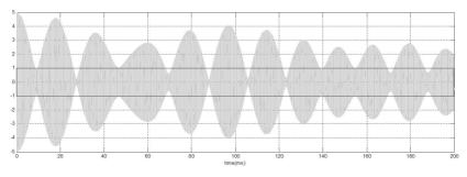
(b) The envelop of the CC-T output in the case of frequency error
