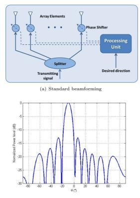
(b) Corresponding beam-pattern to a Uniform Linier Array of 10 antennas
