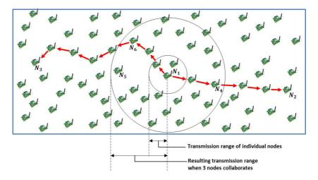
Figure 4.2: Comparison of the number of potential relay nodes in MH and MH-CC (for M = 3 C-nodes)
