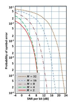
Figure 3.5: Relation of the signal quality to the received SNR and modulation order [PS07]
