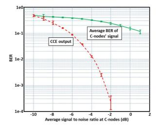
Figure 3.7: Comparison of the signal quality in terms of BER with and without the application of CCE
