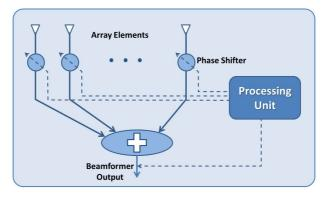
Figure 3.3: The standard structure of receive beamforming
