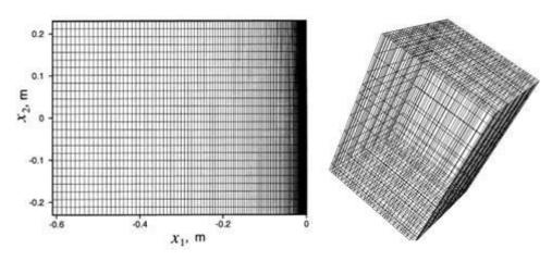
Figure 2.11 2D and 3D computational domains with rectilinear grids
