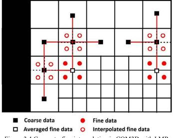
Figure 3.4 Coarse-to-fine interpolation in COM3D with LMR
