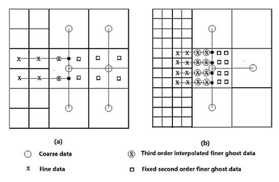
Figure 3.24 Parabolic and linear hybrid interpolation
