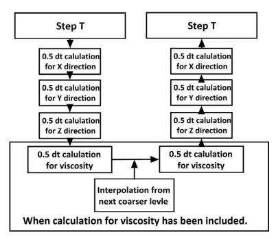
Figure 3.29 One step of AD based solution of NS equations on finer level
