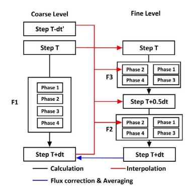
Figure 3.10 RK4 with full-scale LMR in solution of Euler equations
