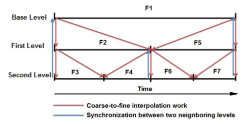
Figure 2.20 Process of Forward Euler scheme with LMR
