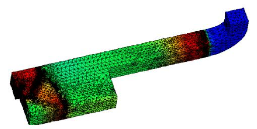
Figure 2.7 Computational domain for detonation simulation in Rut facility [90]
