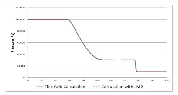
Figure 3.15 Comparison between local mesh refinement and full refinement
