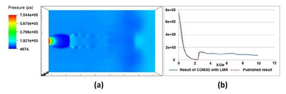
Figure 5.20 Result of pressure in case NPR=7.55
