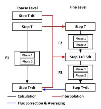
Figure 3.9 RK2 with LMR in the solution of Euler equations
