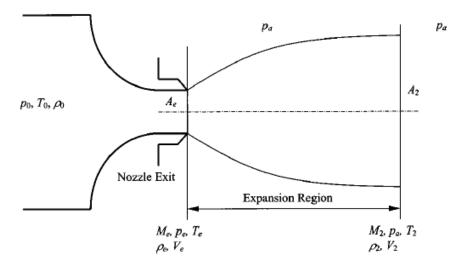
Figure 5.17 Schematic depicting the initial expansion process of an underexpanded jet
