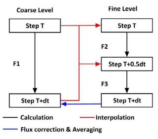
Figure 3.27 The FE based solution of NS equations with LMR
