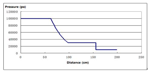
Figure 3.13 Analytical solution of the sod shock tube at T=0.01s
