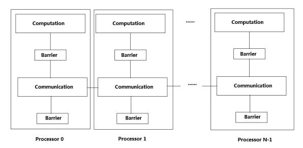
Figure 2.23 One step of parallel computation with N processors
