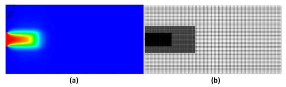
Figure 5.12 Nitrogen mass fraction (a) and grids (b) of the simulation with ALMR at T=0.0108s
