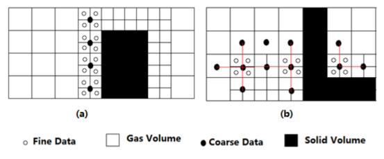
Figure 3.5 Coarse-to-fine data transfer in COM3D
