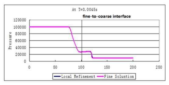
Figure 3.21 Comparison between the local mesh refinement and full refinement in the pressure at T=0.0045s.
