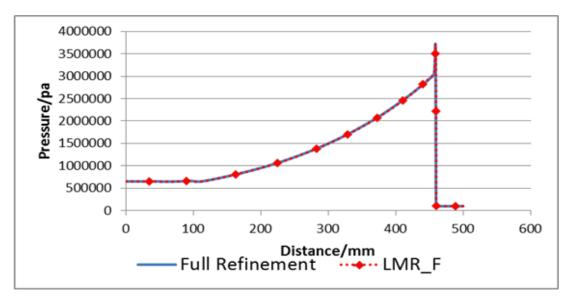
Figure 3.45 Comparison of pressure at T=0.00019s
