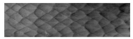
Figure 5.27 cellular structure of detonation wave
