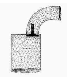
Figure 2.6 Grid structure in ANSYS CFX [2]
