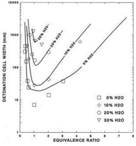
Figure 2.3 Detonation cell width under different initial conditions
