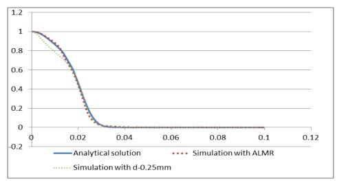
Figure 5.13 Comparison of central line nitrogen mass fractions at T=0.0108s
