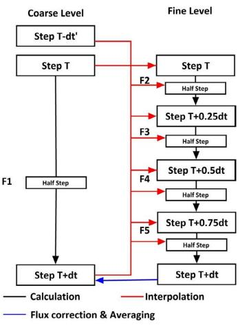
Figure 3.30 AD based solution of NS equations with LMR
