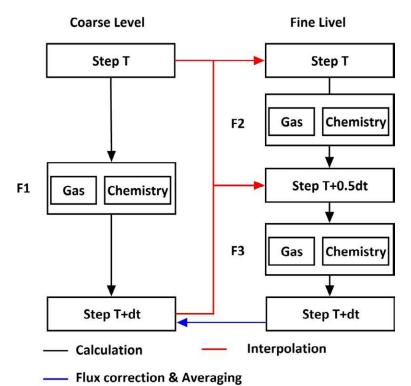
Figure 2.22 Detail process of detonation simulation in two neighbor levels
