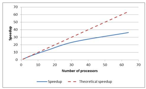
Figure 4.13 Speed up gained by the new decomposition
