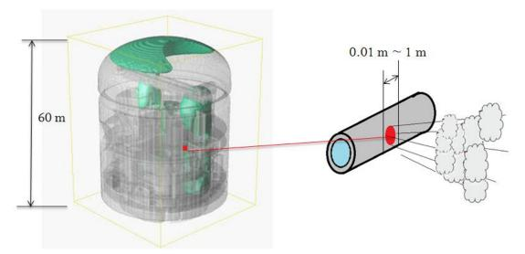
Figure 5.16 Loss Of Coolant Accident (LOCA) inside EPR containment
