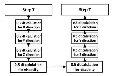
Figure 3.28 One step of AD based solution for NS equations
