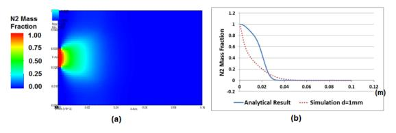
Figure 5.4 Results of simulation with resolution d=1mm
