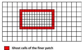
Figure 2.16 Ghost cells on finer levels in domain with patch-based LMR
