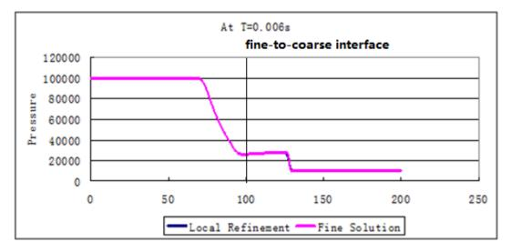
Figure 3.22 Comparison between the local mesh refinement and full refinement in the pressure at T=0.006s.
