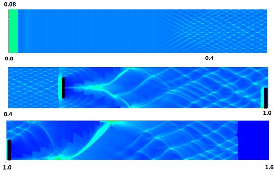
Figure 5.38 Numerical smoke-foil record for simulation with one finer level
