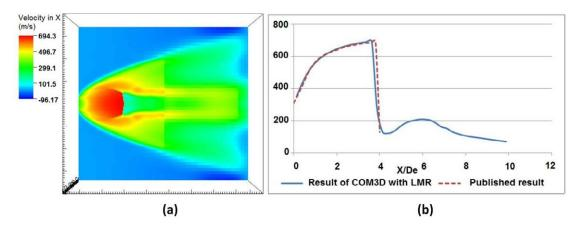
Figure 5.22 Result of velocity in X direction in case NPR=15.53
