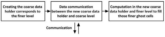
Figure 4.1 Process of coarse-to-fine interpolation
