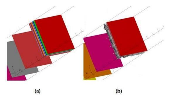
Figure 5.40 Contour figure of  $V_{x}$  in coarse grid (a) and ALMR (b) simulation at step 400  $\,$
