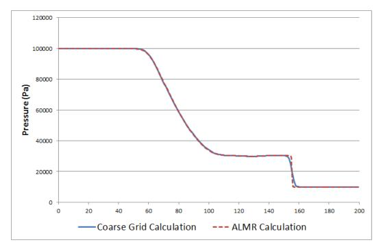
Figure 3.17 Comparison between the simulation with adaptive LMR and coarse grid simulation
