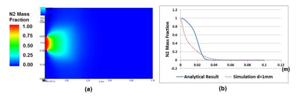
Figure 5.6 Results of simulation with resolution d=0.25mm
