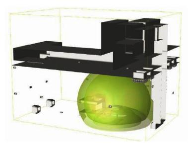
Figure 2.5 Pressure wave resulted from detonation in 160m<sup>3</sup> workshop
