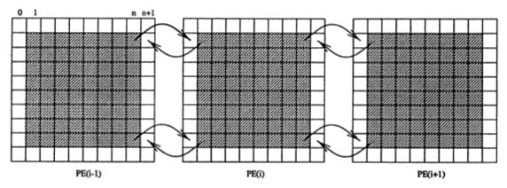
Figure 2.15 Data blocks and data communication in parallel computation
