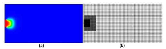
Figure 5.8 Nitrogen mass fraction (a) and grids (b) of the simulation with ALMR at T=0.0036s
