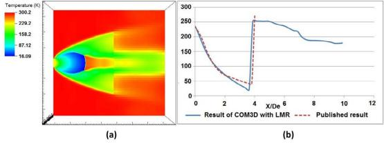
Figure 5.24 Result of temperature in case NPR=15.53
