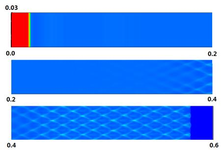
Figure 5.33 Numerical smoke-foil record for 2D detonation with ALMR
