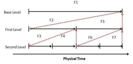
Figure 2.21 Process of forward Euler based detonation simulation with LMR [25]
