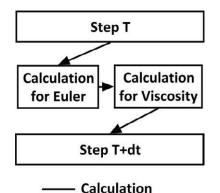
Figure 3.26 One step of FE based solution of NS equations
