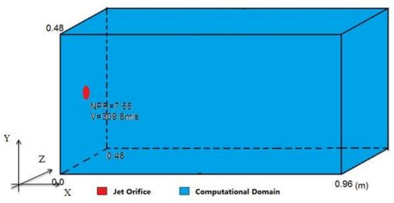
Figure 5.18 Computational domain of the jet simulation
