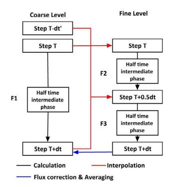
Figure 3.8 AD based solution of Euler equations with LMR
