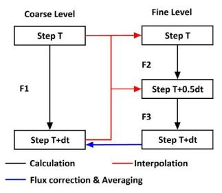
Figure 3.6 FE based solution of Euler equations with LMR
