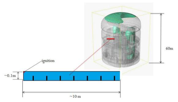
Figure 5.28 Detonation simulation inside EPR containment
