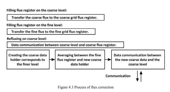
To make the flux correction, 2 sets of flux registers are created on both coarse and fine levels. Those flux registers have the same distribution as the data grids, so the register updating does not require the MPI-based communication. In the refluxing, similarly to the other two communications, the averaging should be done between the finer level and the temporary coarse data holder, and the MPI-based data communication is done between the coarse level and the temporary coarse data holder only.
