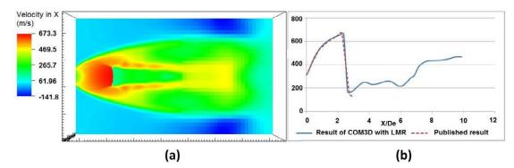
Figure 5.19 Result of velocity in X direction in case NPR=7.55
