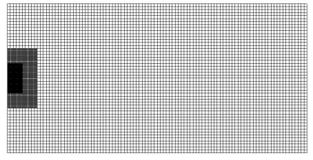
Figure 5.7 Initial grid of the simulation of 2D diffusion
