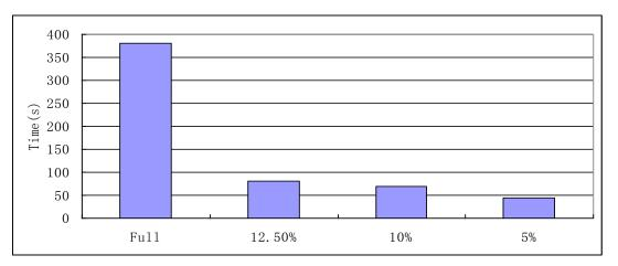
Figure 3.16 Total time cost of the full refinement case and local mesh refinement cases
