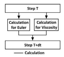
Figure 3.31 One step of calculation for intermediate phase in RK scheme
