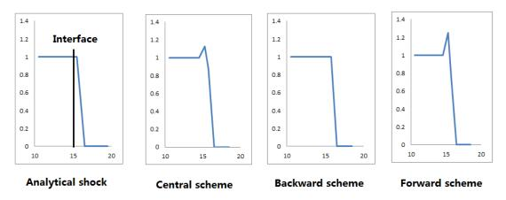
Figure 3.3 Linear interpolation for shock wave in Case 2
