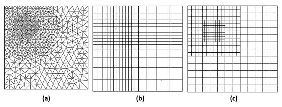
Figure 2.14 Local mesh refinement in with three different approaches
