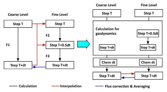
Figure 3.40 First order detonation simulation with further operator splitting
