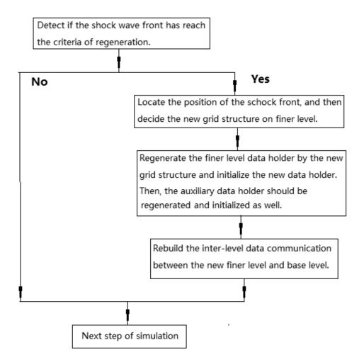
Figure 5.32 Process of re-gridding in detonation simulation
