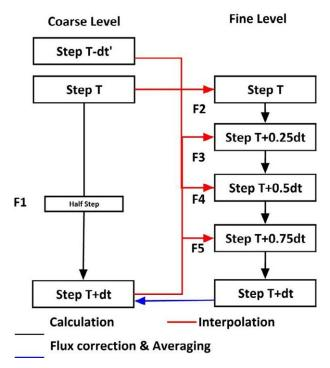
Figure 3.32 RK2 based solution of NS equations with LMR
