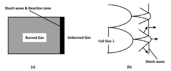
Figure 2.2 Actual structure of a detonation front & Detonation cells
