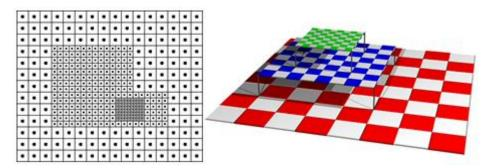
Figure 2.13 Patch-based local mesh refinement
