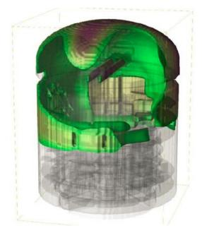
Figure 2.4 Distribution of hydrogen 0.5s after the ignition in EPR containment
