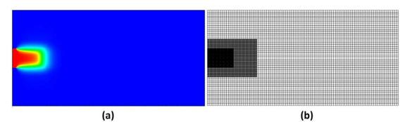
Figure 5.10 Nitrogen mass fraction (a) and grids (b) of the simulation with ALMR at T=0.0072s
