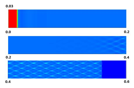
Figure 5.31 Numerical smoke-foil record of the finer case
