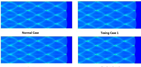
Testing Case 2Testing Case 3Figure 3.39 Simulation of detonation cells in all the testing cases
