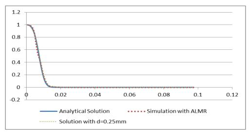
Figure 5.9 Comparison of central line nitrogen mass fractions at T=0.0036s
