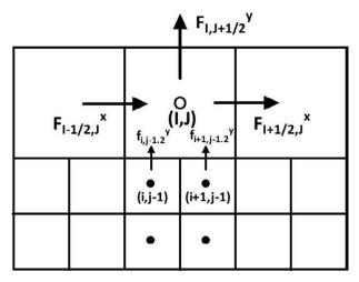
Figure 2.19 Fluxes on the fine-to-coarse interface
