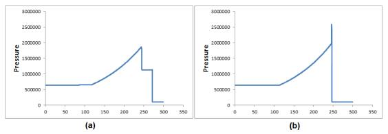
Figure 1.4 1D detonation simulation with resolution 0.1m (a) showing unphysical step structure and finer resolution 0.001m (b) showing proper physical behavior
