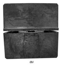
**Figure 4.6.** – Brass inlay for the sharkskin die-1, applied on the sharkskin die-1. (a) brass inlay inserted in the opened die. (b) front view of the closed sharkskin die-1 with brass inlay with a slit cross-section of 10 mm  $\times$  2 mm.
