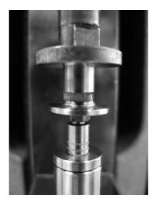
**Figure 5.6.** – The newly designed axial force measurement device for the CaBER with a sample loaded. The plates have a diameter of 6 mm. The lower plate geometry is directly screwed into the force transducer and fixed with a counter nut.
