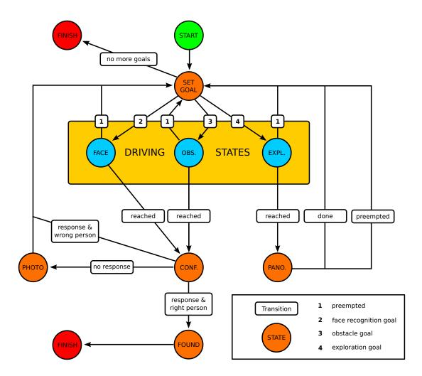
Figure 4.14: The state machine of the search process. The states are explained in table 4.2.
