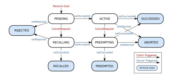
Figure 3.4: States and transitions of goals on the side of an actionlib server (taken from [ros14a])
