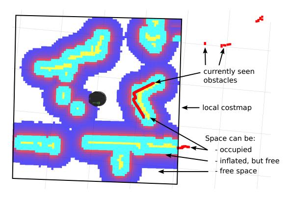
Figure 4.7: Visualization of the incoming data in RViz. The local costmap around the robot is marked by a rectangle. Occupied points are shown in yellow. Free space is white and all other colors are information for the navigation cost function but represent free space [ros14c]. The currently seen occupied points are marked in red and go further than the costmap.
