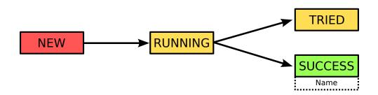
Figure 4.13: The states of obstacle and face detections. First all detections are unconfirmed, then an external process can report an ongoing confirmation. This can result in success or fail. A successful confirmation can assign to a detection.
