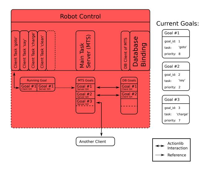
Figure 4.5: Detailed view on the robot control structure. The upper half shows the server and clients and the lower half the corresponding data structures for the goal storage. The database submitted two goals and another client the goal #3. Goal #1 is running on the task server of the task 'goto'.
