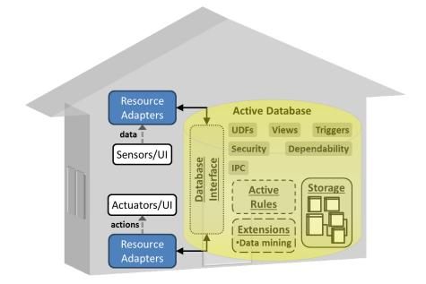
Figure 2.1: The proposed architecture of an active database in a smart home. Every resource is connected through a resource adapter. The active database components are examined in and the figure is taken from [dMW13].
