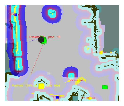
Figure 5.4: A running exploration task. The blue and red line are the planned navigation trajectories. In the bottom left the representation of a recognized face can be seen. In the bottom middle a detected but low rated obstacle can be seen.
