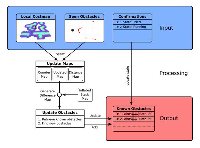
Figure 4.9: Process flow of one cycle in the obstacle approach
