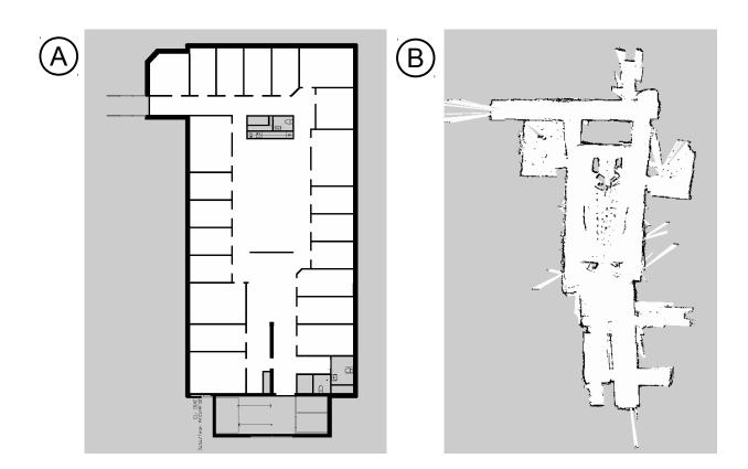
Figure 4.2: A: occupancy map based on the floor plan B: a map created with the gmapping SLAM implementation<sup>3</sup>
