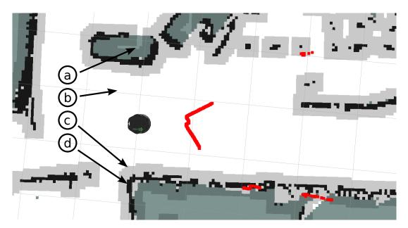
Figure 4.8: The static map and the inflated map overlayed in RViz.
