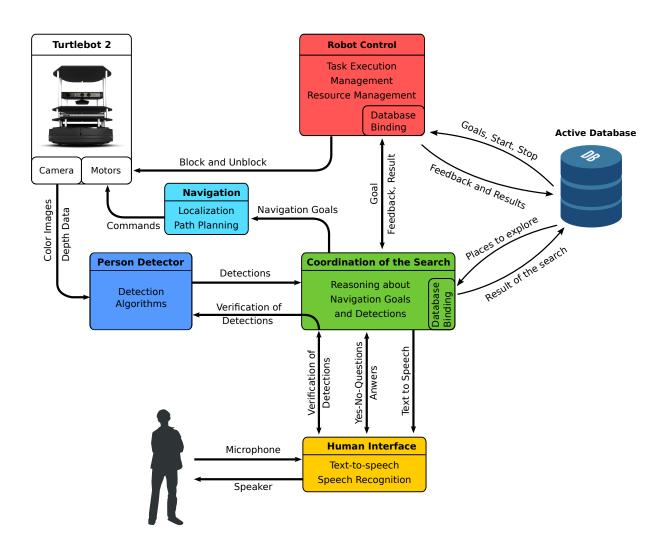
Figure 4.1: Simplified overview of the hardware and software components
