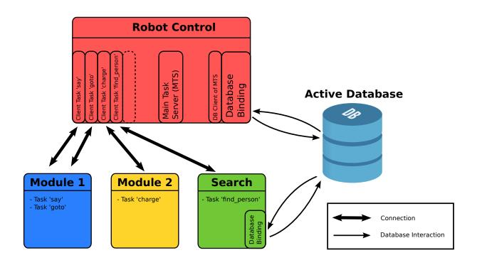
Figure 4.4: The design concept of the robot control software. Module 1 can execute two different tasks. Module 2 offers one task. The module 'search' can execute one task and has an own database connection.
