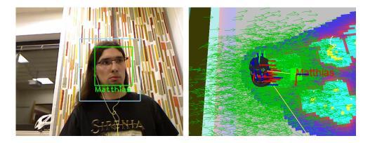
Figure 4.10: The left picture shows a detected head (outer blue rectangle) and the detected face within the head (inner green rectacle) with the assigned name. On the right picture the published coordinate frame as well as the visualization in RViz can be seen. (On the ground the local costmap as well as the localization assumptions are displayed)
