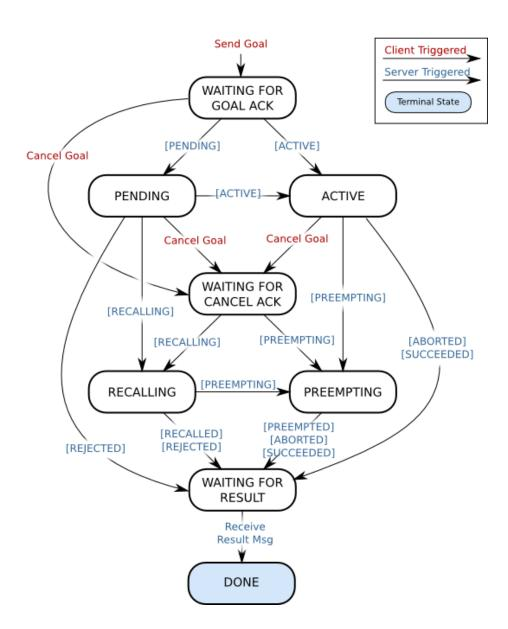
Figure 3.3: States and transitions of goals on the side of an actionlib client (taken from [ros14a])
