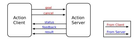
Figure 3.2: The interface between an actionserver and an actionclient
