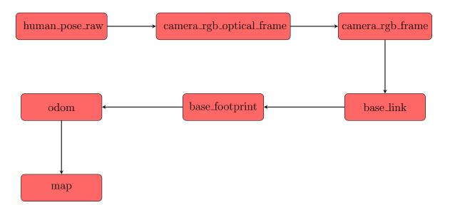
Figure 4.12: Transformation chain between a detection and the coordinate frame of the map.
