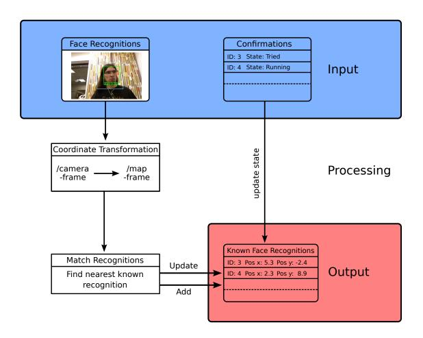
Figure 4.11: One cycle in the face detection.
