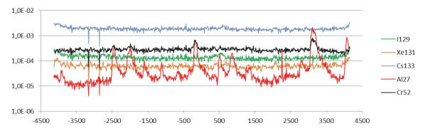
*Figure 11:* Ablation profiles on sample C1 at the  $4^{th}$  passage in the track marked 1 in Figure 9 (60  $\mu$ m beam).
