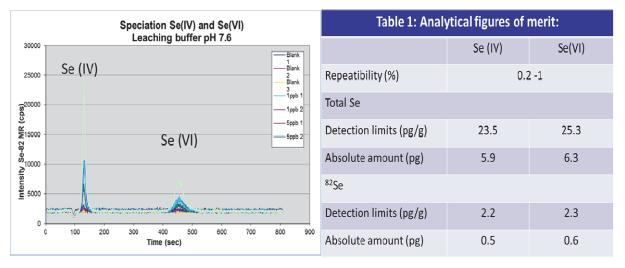
Figure 8:. (A) Se species elution profiles at different concentrations. (B) Analytical figures of merit.
