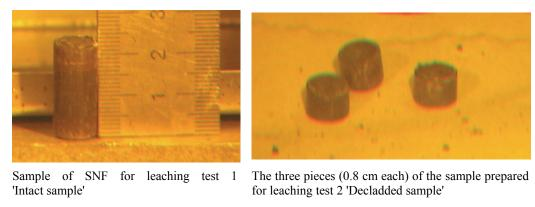
Figure 1: Samples prepared for the two leaching tests with spent nuclear fuel.
