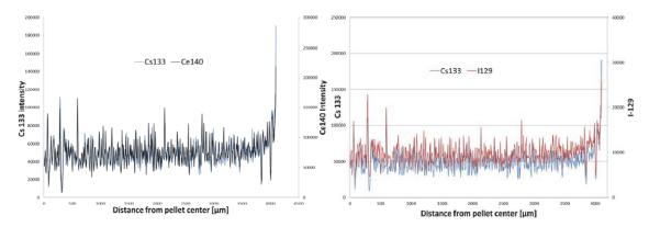
**Figure 8:** Ablation profiles on 5A2 along the yellow dotted track in figure 5. Left, overlaid Cs-133 & Ce-140 profiles. Right, overlaid Cs-133 & I-129 profiles (10 µm beam).
