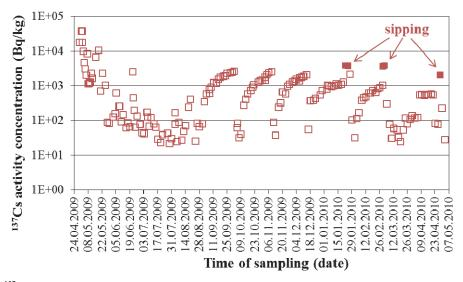
Figure 3: History of <sup>137</sup>Cs activity concentration in the spent fuel storage pool of Unit 4.
