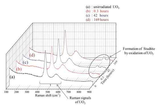
Figure 3: Raman spectra of unirradiated  $UO_2$  ((a)) and a sample irradiated at 8.73 kGy under open atmosphere ((b), (c) and (d)). The spectra (b), (c) and (d) are obtained 0.3, 42 and 169 hours after contact with the irradiated solution.
