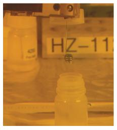
Figure 2: SNF sample suspended in a Pt wire.
