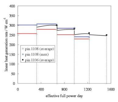
Figure 2: Power history of fuel rod 1106 (average LHGR; after Stratton et al., 1991) compared to average and maximum LHGR data of fuel rod SBS1108.
