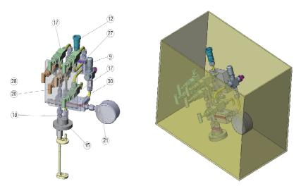
Figure 1: Design of autoclave head (left) and the tested dimension of the head in the hot cell conveyer container (right).
