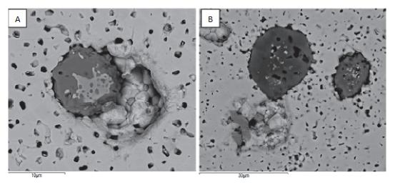
**Figure 1:** A: SEM-BS image of a typical oxide precipitate present in the low-doped sample; B: Different type of secondary phases in the highly doped SIMFuel sample.
