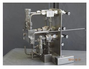
Figure 2: Manufactured autoclave head.
