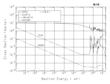
Figure 1: Point-wise cross-sections from JENDL-3.2 (taken from www.nuclides.net).
