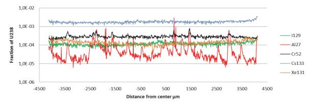
Figure 12: Ablation profiles on sample C1 along the track marked 2 in Figure 9 (60 µm beam).
