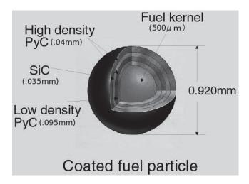
Figure 1: Design of a TRISO coated fuel particle.
