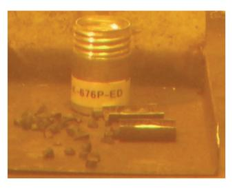
Figure 6: Sample KKG-13-5024-10-K-676-ED after cutting and defueling (sample type: fuel fragments).
