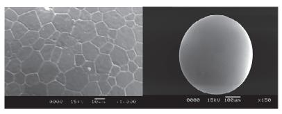
Figure 1: SEM picture of the surface of an unirradiated  $UO_2$  particle.
