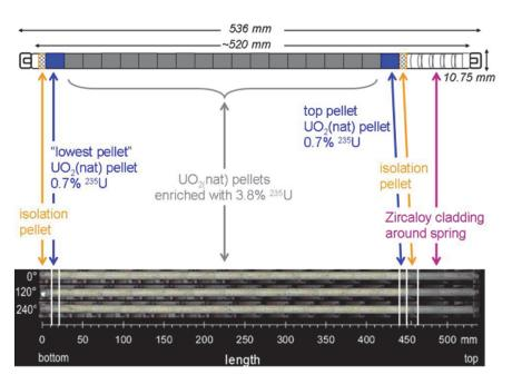
Figure 1: Schematic cross section and photos of the fuel rod segment SBS1108-N0204. The inserted photo is taken from Papaioannou et al. (2012).
