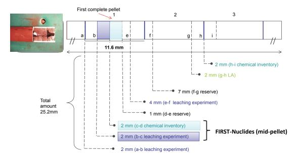
**Figure 4:** BWR42 cutting plan showing the position and the nominal length of samples cut mid-pellet for IRF leaching studies and for further characterisations (solid vertical lines indicate pellet-pellet gaps; dashed lines indicate cut positions).
