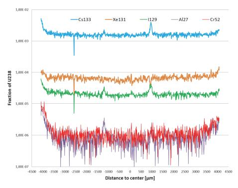
Figure 6: Ablation profiles on 5A2 along the red dashed track in figure 5 (60 µm beam).
