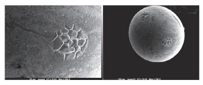
Figure 2: SEM pictures of the surface of a  $UO_2$  particle corroded in open air atmosphere.
