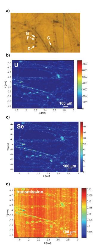
Figure 3: Optical microscope (a),  $\mu$ -XRF maps corresponding to the U (b) and Se (c) fluorescence signals and transmitted intensity (d) of a section in the middle region of the dispersed UO<sub>2</sub> spent fuel sample investigated in May 2013. Letters and arrows in the microscopic image denote locations where Se K-edge XANES spectra were recorded. Map coordinates are in mm. Color coding represents detector counts (b, c) and voltages of the diode (d) used to measure the transmitted signal.
