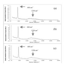
Figure 1: Micro-Raman spectra of an undoped  $UO_2$  sample: (a) as received; and after 1 h exposure to (b) oxygenated water and (c) 100  $\mu$ mol/dm<sup>3</sup>  $H_2O_2$
