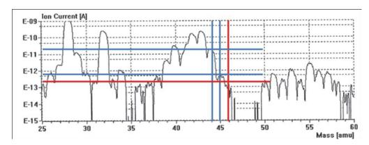
Figure 3: Measured  $^{12}CO_2$  (blue),  $^{13}CO_2$  (blue), and  $^{14}CO_2$  (red) signals in the gas sampled from the plenum of KIT's SNF rod (analysed with a quadrupole gas mass spectrometer (GAM400, In Process Instruments).
