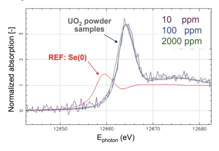
Figure 7: Se K-edge XANES of the three doped non-irradiated  $UO_2$  powdered samples listed in Table 1, compared to the Se K-edge spectrum of a metallic Se reference.
