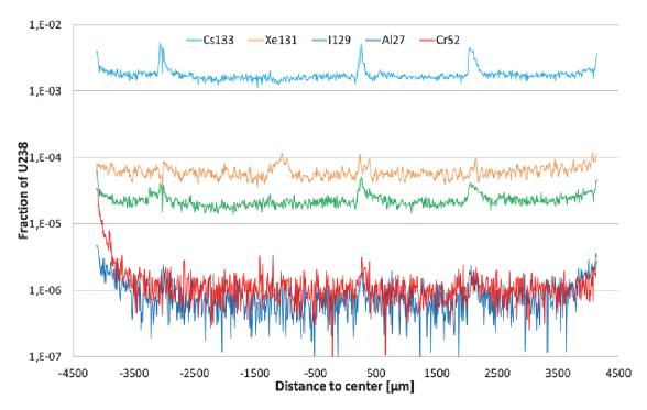
Figure 7: Ablation profiles on 5A2 along the green track in figure 5 (60  $\mu$ m beam).
