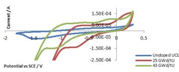
**Figure 4:** Cyclic Voltammogram of Undoped  $UO_2$ , 25 GWd/ $t_U$  and 43 GWd/tU SIMFUEls in modified simplified Groundwater, sparged with Argon.
