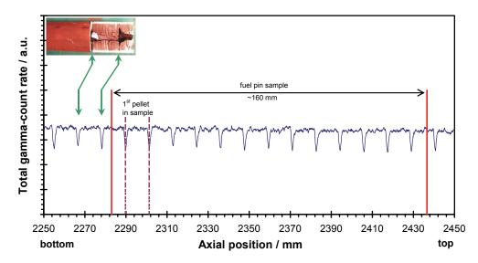
Figure 3:  $\gamma$ -scan of BWR42 illustrating the location of the fuel pin sample and showing the pellet positions in the sample (see also the macrograph of the axially cut open pin in the upper left corner).
