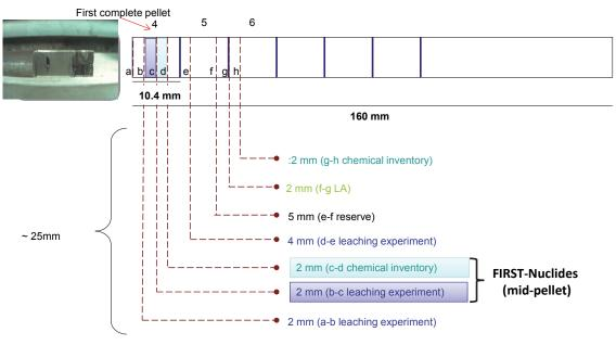
**Figure 5:** BWR54 cutting plan showing the position and the nominal length of samples cut mid-pellet for IRF leaching studies and for further characterisations (solid vertical lines indicate pellet-pellet gaps; dashed lines indicate cut positions).
