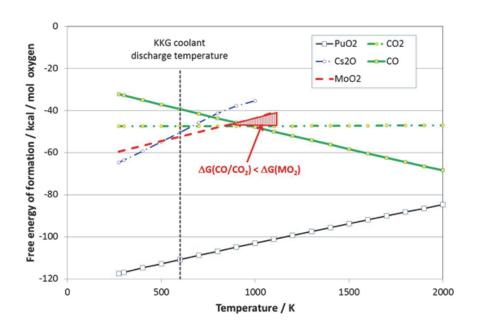
Figure 2: Free energy of formation for carbon oxides,  $Cs_2O$ ,  $MoO_2$  and  $PuO_2$ . The vertical dashed line indicates approximately the surface temperature of the cladding, the red triangle shows the temperature region where  $\Delta G_f$  of the carbon oxides are below those of  $MoO_2$ .
