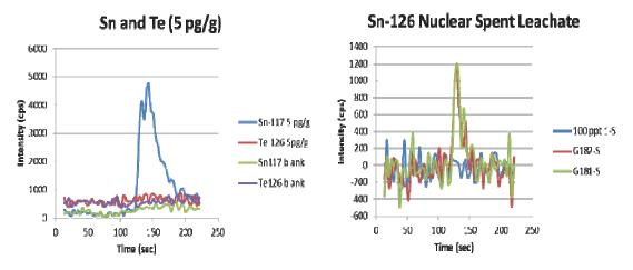
Figure 9:. (A) Behaviour of Sn and Te in the chelating column. (B) Detection of 126 Sn in nuclear spent fuel leachates (dilution 1/10).
