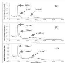
Figure 2: Micro-Raman spectra of a 25 GWd/tU SIMFUEL sample: (a) as received; and after 1 h exposure to (b) oxygenated water and (c) 100  $\mu$ mol/dm<sup>3</sup>  $H_2O_2$
