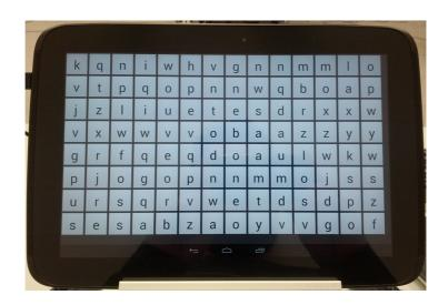
Figure 4.41: The Nexus 10 tablet used in the user study, displaying buttons of the same size with random letters as labels.
