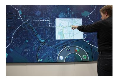
Figure 5.5: A map overlay can be freely moved across the video wall by pointing to the desired location. A click discards the tool.
