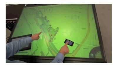
Figure 5.8: By pointing to the map on the digital situation table and the smartphone as well, the map data from the table is automatically transferred to the smartphone.
