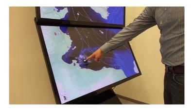
Figure 5.16: The fingertip detector works up to the displays surface and allows pointing as well as touch interaction.
