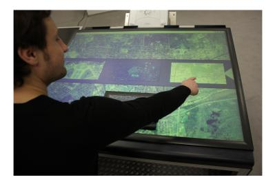
Figure 5.7: A hand gesture consisting of a single, streched out finger allows to trigger clicks and choose between different map layers, for example.
