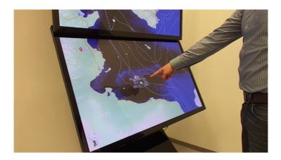
Figure 5.15: A fingertip detector allows pointing interaction with a single finger, accurate enough to select small items such as individual boats.
