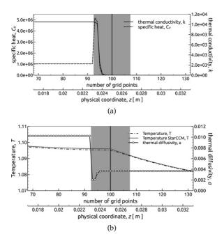
**Figure 6.11:** Inverse/harmonic interpolation in *k* and factorised inverse/harmonic interpolation of  $C_V$  using a phase dependent decaying factor. (a) interface profile  $\phi$  together with material properties *k* and  $C_V$ , (b) temperature profile, interface profile  $\phi$  and thermal diffusivity *a*. The shadowy area indicates the diffuse interface region, with a vertical line at  $\phi = 0.5$ .
