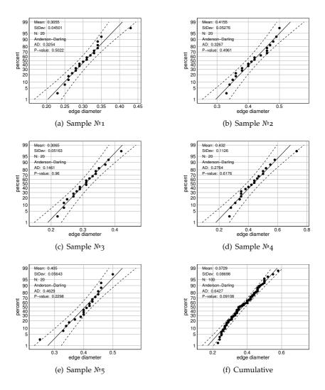
**Figure A.11:** Normal probability plots of edge thickness, (a)-(e) of the individual 30 ppi aluminium samples 1-5 and (f) cumultative normal probability plot.
