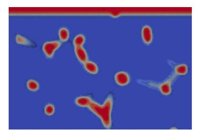
**Figure 7.8:** Distribution of the order parameter on a longitudinal cross section through the computational domain. The blue regions indicate fluid, the red regions solid and the diffuse interface is highlighted by showing the corresponding cells in case of non vanishing gradients of the order parameter.
