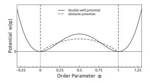
**Figure 4.2:** Course of the terms for the *obstacle* and *double-well* potential. Whereas the stable states are located in the minima of the double-well potential, the obstacle is defined on the Gibbs-Simplex.
