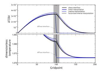
**Figure 6.14:** Temporal temperature difference and the dimensionless temperature profiles for a 1D simulation of a equally spaced composite domain (aluminium/air) heated from one side, for the linear interpolation, the inverse interpolation and the factorised inverse interpolation of  $C_V(\phi)$  in the diffuse interface compared to the sharp interface solution.
