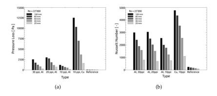
**Figure 3.25:** Comparison of (a) pressure loss and (b) heat transfer characteristics of different foam types and cylindrical reference samples of different lengths at a Reynolds number of approximately Re  $\approx 22'000$ .
