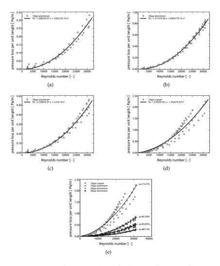
**Figure 3.18:** Pressure loss per unit length for (a) 10 ppi aluminium, (b) 20 ppi aluminium, (c) 30 ppi aluminium, (d) 10 ppi copper and (e) comparison of all foam types. The black solid line represents a quadratic fit of type  $y = a x^2 + b x$ . Samples of the same pore density are combined for overall lengths from 20 mm to 100 mm.
