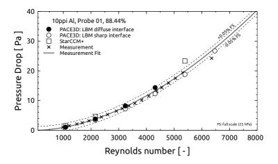
**Figure 7.9:** Comparison of measured and simulated pressure loss data. An additional measurement series is performed for low to medium Reynolds numbers using a high accuracy pressure transducer. The level of accuracy is indicated by the upper and lower error limits at  $\pm 0.05$ %. The results of StarCCM are shown as a reference, whereas *sharp interface* as well as *diffuse interface* results are given for PACE3D.
