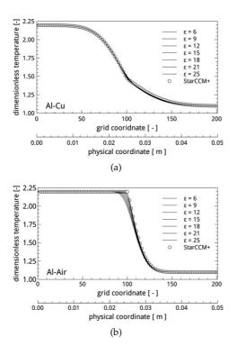
Figure 6.17: 1D heat conduction perpendicular to the interface for for different widths of the diffuse interface for (a) aluminium-copper and (b) aluminium-air.
