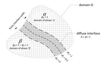
**Figure 4.1:** Scheme of a computational domain  $\Omega$  with phases  $\alpha$  and  $\beta$ . Utilising the phase field method, the interface is of finite width, and the order parameter  $\phi_{\alpha}$  changes from 1 to 0 across the diffuse interface, whereas  $\phi_{\beta} = 1 - \phi_{\alpha}$ . The order parameters  $\phi_{\alpha}$  and  $\phi_{\beta}$  as well as the characteristic properties of the individual phases are constant throughout the bulk areas, respectively.
