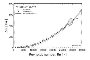
**Figure 7.5:** Comparison of experimental and numerical pressure loss data obtained with StarCCM for the 10 ppi aluminium foam sample  $N^{\circ}1 \psi = 88.44\%$  of length 20 mm.
