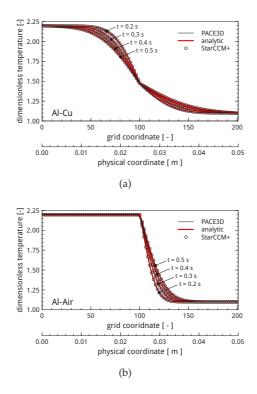
**Figure 6.16:** One dimensional heat conduction perpendicular to interface for (a) aluminium-copper and (b) aluminium-air for different instances of time.
