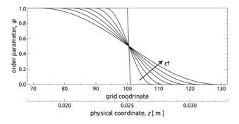
Figure 6.3: Phase-field profile shape for different interface widths.
