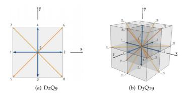
**Figure 5.1:** Unit lattice of the discrete velocities for (a) the two dimensional D2Q9 model and (b) the three dimensional D3Q19 model. In the unit lattice, the vectors have discrete directions as well as discrete magnitudes. For the models depicted, the vectors can have three magnitudes: o for particles at rest (centered at the origin of the unit lattices), 1 for particles travelling parallel to the axis (blue),  $\sqrt{2}$  for particles travelling along plane diagonal (orange).
