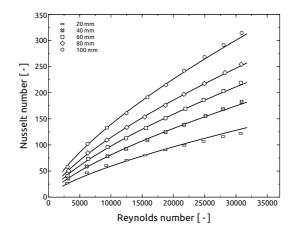
**Figure 3.24:** Nusselt number distributions of the reference samples of lengths 20 mm, 40 mm, 60 mm, 80 mm and 100 mm, measured at 90 °C respectively. The solid lines represent regression curves of type  $Nu = C \cdot Re^{0.7} \cdot Pr^{1/3}$ , for which the coefficients *C* are fitted individually.
