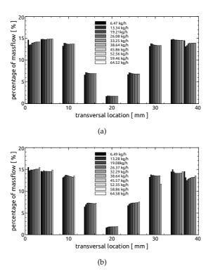
**Figure C.6:** Massflow distribution along transversal direction for 30 ppi aluminium foam of 100 mm length at (a) inlet and (b) outlet.
