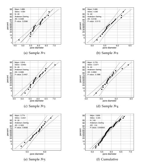
**Figure A.4:** Normal probability plots of pore diameter, (a)-(e) of the individual 10 ppi copper samples 1-5 and (f) cumultative normal probability plot.
