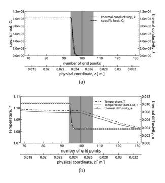
**Figure 6.6:** Inverse/harmonic interpolation in *k* and in *C*<sub>V</sub>. (a) interface profile  $\phi$  together with material properties *k* and *C*<sub>V</sub>, (b) temperature profile, interface profile  $\phi$  and thermal diffusivity *a*. The shadowy area indicates the diffuse interface region, with a vertical line at  $\phi$  = 0.5.
