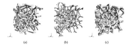
**Figure 7.2:** Different artificially generated foam structures with different porosities, to represent 10 ppi aluminium foams: (a)  $\psi_{\text{modelling}} = 88.44 \%$  corresponding to sample  $N_{2}$  and (c)  $\psi_{\text{modelling}} = 83.85 \%$  corresponding to sample  $N_{2}$  and (c)  $\psi_{\text{modelling}} = 83.85 \%$  corresponding to sample  $N_{2}$ , cf. tab. 7.1.
