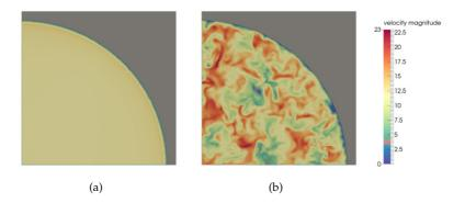
**Figure 7.12:** Distribution of velocity magnitude (a) up- and (b) downstream of the foam sample for a Reynolds number of about  $\text{Re} \approx 26'000$ .
