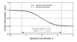
**Figure 4.3:** Steady state solutions of the phase field equations employing the double-well and obstacle potential, respectively. The interface width  $\lambda = \varepsilon \pi^2/4$  is exact for the obstacle potential, whereas for the double-well potential it is defined as 95% of the bulk value of  $\phi$ .
