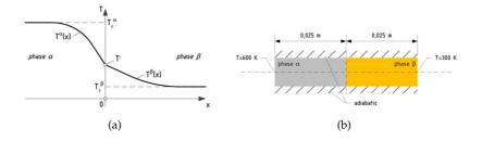
**Figure 6.15:** (a) One dimensional validation of heat conduction for two semi infinite phases  $\alpha$  and  $\beta$ , with initial temperatures  $T_0^{\alpha}$  and  $T_0^{\beta}$  respectively, and (b) setup for the numerical test case.
