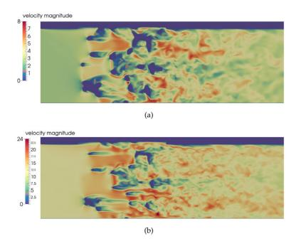
**Figure 7.17:** Velocity distribution on a longitudinal cross section for (a) a Reynolds number of about 6'000 and (b) 26'000 for a 10 ppi aluminium foam sample with porosity  $\psi = 88.44$  %.
