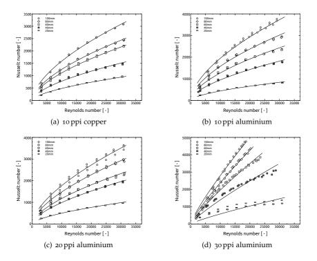
**Figure 3.21:** Nusselt number distributions of all foam types and lengths, each measured at three temperatures, 60 °C, 90 °C and 120 °C, respectively. The solid lines represent correlation curves of type Nu =  $C \cdot \text{Re}^m \cdot \text{Pr}^{1/3}$ , for which the coefficients *C* are evaluated individually, whereas the exponents *m* are constant for each foam type; parameters are tabulated in tab. 3.5.
