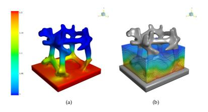
**Figure 7.19:** Temperature distributions on a wall-mounted open cell metal foam with constant wall temperature: (a) temperature distribution on the ligaments of the aluminium foam (b) temperature distribution and isolines on an imprinted transparent cube.
