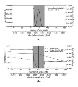
**Figure 6.7:** Inverse/harmonic interpolation in *k* and evaluation of  $C_V$  by linear/direct interpolation of thermal inertia *I*. (a) interface profile  $\phi$  together with material properties *k* and  $C_V$ , (b) temperature profile, interface profile  $\phi$  and thermal diffusivity *a*. The shadowy area indicates the diffuse interface region, with a vertical line at  $\phi = 0.5$ .
