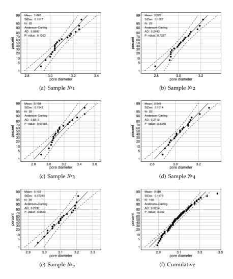
**Figure A.3:** Normal probability plots of pore diameter, (a)-(e) of the individual 30 ppi aluminium samples 1-5 and (f) cumultative normal probability plot.
