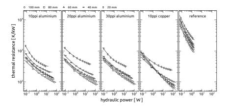
**Figure 3.26:** Thermal resistance vs. hydraulic power for all foam types and lengths in comparison to the tubular reference probe.
