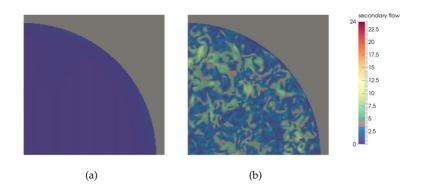
**Figure 7.15:** Velocity distribution of the secondary flow structure (a) up- and (b) downstream of the foam sample for a Reynolds number of about  $\text{Re}\approx6'000$ .
