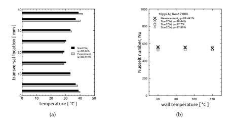
**Figure 7.6:** Exemplary thermal results of fluid flow and heat transfer simulation of open cell metal foam using StarCCM: (a) comparison of measured and simulated temperature profile in the outflow and (b) comparison of measured and simulated Nusselt numbers at three different temperature levels ( $60^{\circ}C$ ,  $90^{\circ}C$  and  $120^{\circ}C$ ) for foams of comparable porosity.
