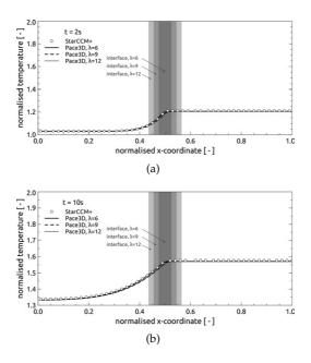
**Figure 6.24:** Temperature profiles across the parallel interface after (a) two seconds and (b) ten seconds, each compared to the numerical reference solution obtained with StarCCM. The shadowy region marks the diffuse interface layer.
