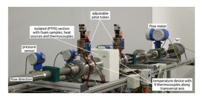
Figure 3.12: Final installation of the test rig.
