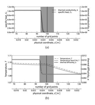
**Figure 6.8:** Inverse/harmonic interpolation in *k* and evaluation of  $C_V$  by inverse/harmonic interpolation of thermal inertia *I*. (a) interface profile  $\phi$  together with material properties *k* and  $C_V$ , (b) temperature profile, interface profile  $\phi$  and thermal diffusivity *a*. The shadowy area indicates the diffuse interface region, with a vertical line at  $\phi = 0.5$ .
