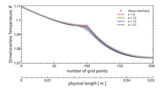
**Figure 6.12:** Interpolation of material properties *k* and  $C_V$ , interpolation of thermal diffusivity *a* and temperature profile, using decaying factorised inverse/harmonic interpolation in  $C_V$  for different diffuse interface widths,  $\epsilon$ .
