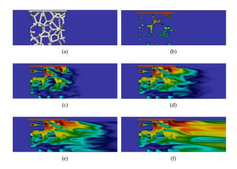
**Figure 7.22:** Time series of unsteady temperature distributions on a longitudinal cross section. Here, the foam structure depicted in (a) is subject to a radial initial temperature distribution (b). The figs. (c) to (f) give an impression of the temporal evolution of the temperature field.
