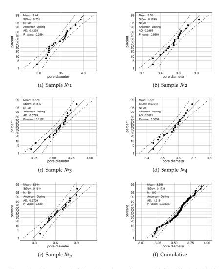
**Figure A.2:** Normal probability plots of pore diameter, (a)-(e) of the individual 20 ppi aluminium samples 1-5 and (f) cumultative normal probability plot.
