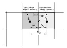
Figure 6.1: Sharp interface finite volume example.
