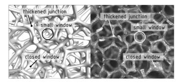
**Figure 7.1:** Pore scale features (small window, closed window and thickened junctions) of artificial and real foam structures.
