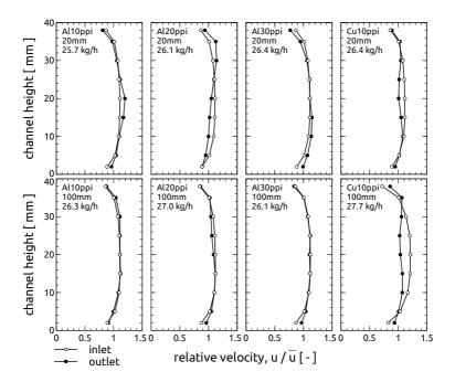
**Figure 3.23:** Relative velocity distributions at inlet and outlet of all foam types for 20 mm and 100 mm length, respectively.
