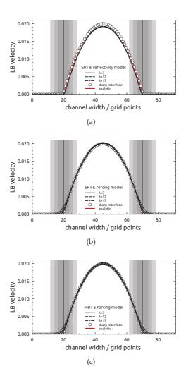
**Figure 5.3:** Comparison of velocity profiles of the plain Poiseuille flow obtained analytically, with sharp interface with different diffuse interface and lattice models: (a) SRT lattice BGK model and *reflectivity* model (b) SRT lattice BGK model and *forcing* model (c) MRT lattice Boltzmann model and *forcing* model. The shadowy regions mark the diffuse interface layer.
