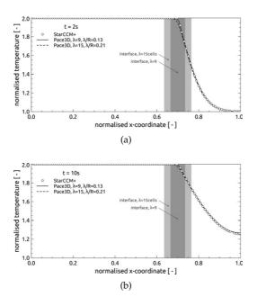
**Figure 6.22:** Temperature profiles across the convex interface (circular inclusion of aluminium in air) for long-time simulations (a) for 2 s and (b) for 10 s, using the segmented approach, each compared to the numerical reference solution obtained with StarCCM. The shadowy regions mark the diffuse interface layer.
