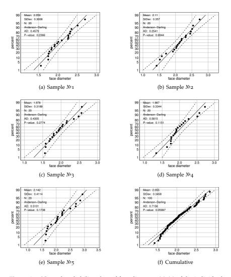
**Figure A.8:** Normal probability plots of face diameter, (a)-(e) of the individual 10 ppi copper samples 1-5 and (f) cumultative normal probability plot.
