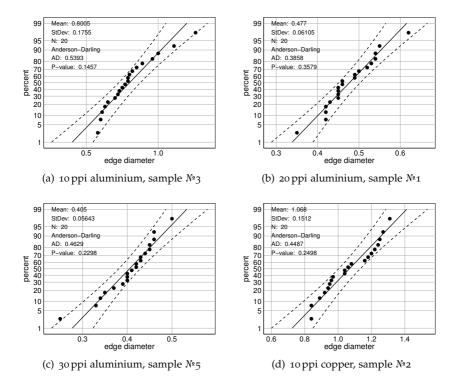
**Figure 3.5:** Exemplary normal probability plots of the measured edge thickness for (a) 10 ppi aluminium sample  $N_2$  (b) 30 ppi aluminium sample  $N_2$  (c) 20 ppi aluminium sample  $N_2$  and (d) 10 ppi copper sample  $N_2$ . The dotted lines represent the 95 % confidence interval, respectively.
