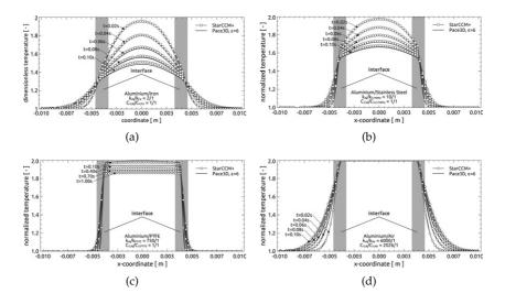
**Figure 6.18:** Comparison of the temperature distributions for a two dimensional circular inclusion at a horizontal cross section obtained with PACE3D and Star-CCM for different instances of time and for material combinations (a) aluminium/iron, (b) aluminium/stainless steel, (c) aluminium/PTFE, (d) aluminium/air. The shadowy regions mark the diffuse interface layer.
