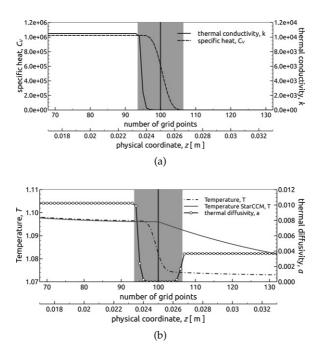
**Figure 6.5:** Inverse/harmonic interpolation in *k* and direct/arithmetic interpolation in  $C_V$ . (a) interface profile  $\phi$  together with material properties *k* and  $C_V$ , (b) temperature profile, interface profile  $\phi$  and thermal diffusivity *a*. The shadowy area indicates the diffuse interface region, with a vertical line at  $\phi = 0.5$ .
