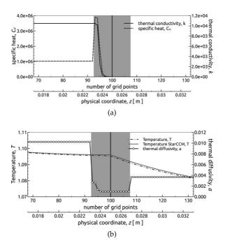
**Figure 6.9:** Inverse/harmonic interpolation in *k* and factorised inverse/harmonic interpolation of  $C_V$  using a single fixed factor. (a) interface profile  $\phi$  together with material properties *k* and  $C_V$ , (b) temperature profile, interface profile  $\phi$  and thermal diffusivity *a*. The shadowy area indicates the diffuse interface region, with a vertical line at  $\phi = 0.5$ .
