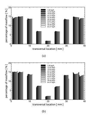
**Figure C.1:** Massflow distribution along transversal direction for 10 ppi aluminium foam of 20 mm length at (a) inlet and (b) outlet.
