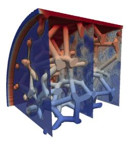
**Figure 7.20:** Temperature distribution inside a 10 ppi aluminium foam sample of porosity  $\psi = 88.44$  %. The temperature is given on the surface of the foam structure as well as on three lateral cross sections for the fluid, where low and high temperature corresponds to blue and red colours, respectively.
