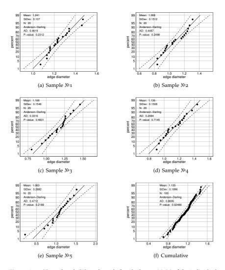
**Figure A.12:** Normal probability plots of edge thickness, (a)-(e) of the individual 10 ppi copper samples 1-5 and (f) cumultative normal probability plot.
