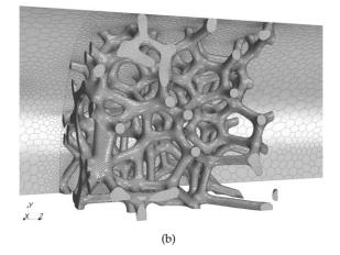
**Figure 7.4:** Exemplary polyhedral mesh in StarCCM, with about  $8.4 \times 10^5$  elements: (a) longitudinal cross section and (b) solidsurface representation of the computational domain with  $8.4 \times 10^5$  cells,  $4.9 \times 10^6$  faces and  $4.5 \times 10^6$  vertices.
