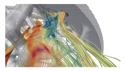
**Figure 7.18:** Visualisation of the flow inside the foam structure with threedimensional streamlines at a Reynolds number of about 26'000. Besides straight flow paths, detached flow is identified in the wake of a foam edge. Streamlines are coloured by the magnitude of the velocity.
