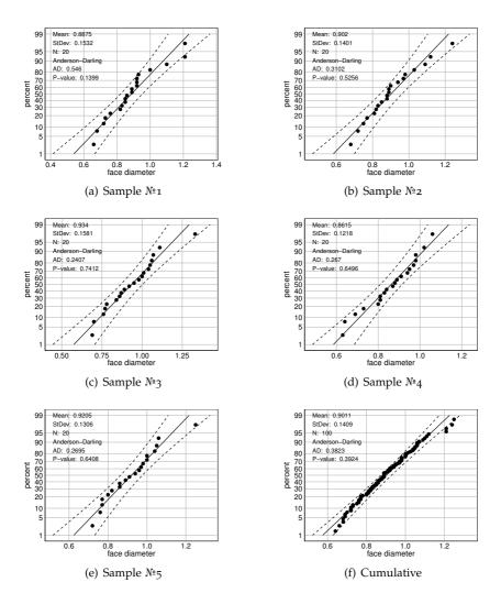
**Figure A.7:** Normal probability plots of face diameter, (a)-(e) of the individual 30 ppi aluminium samples 1-5 and (f) cumultative normal probability plot.
