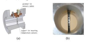
**Figure 3.10:** Detailed view on (a) the three dimensional design model of the custom made temperature probe section of the test rig and (b) the temperature rake inside the probe section.
