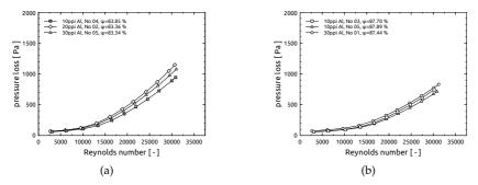
**Figure 3.16:** Pressure loss of foams of similar porosity (a)  $\psi \approx 83\%$  and (b)  $\psi \approx 87\%$ . Reynolds number is based on inlet diameter.
