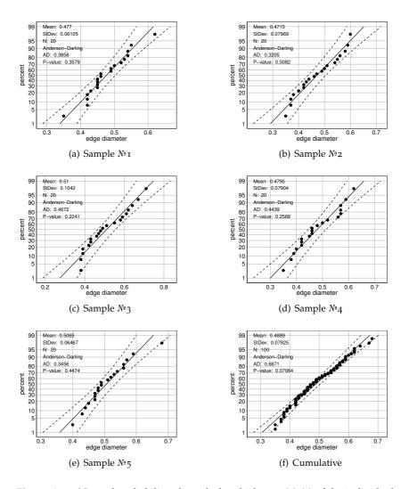
**Figure A.10:** Normal probability plots of edge thickness, (a)-(e) of the individual 20 ppi aluminium samples 1-5 and (f) cumultative normal probability plot.
