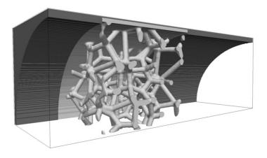
**Figure 7.7:** Computational domain of  $200 \times 200 \times 600$  cells used in PACE3D. The foam is depicted as light greyish surface, whereas the dark grey region indicates the outer solid margin that is defined as a so called barrier region which does not account for the numerical computation.
