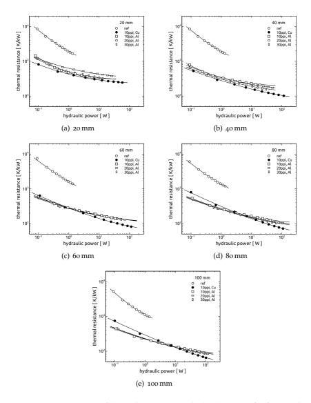
**Figure 3.27:** Comparison of thermal resistance vs. hydraulic power for foam and reference samples of equal lengths 20 mm to 100 mm, (a) to (e), respectively.
