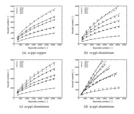
**Figure 3.20:** Nusselt number distributions of all foam types and lengths, each measured at three temperatures, 60 °C, 90 °C and 120 °C, respectively. The solid lines represent correlation curves of type Nu =  $C \cdot \text{Re}^m \cdot \text{Pr}^{1/3}$ , for which the coefficients *C* and exponents *m* are individually fitted for each length; values are tabulated in tab. 3.4.
