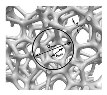
Figure 2.2: Characteristic measures of foams.
