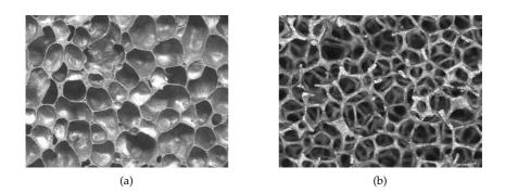
**Figure 2.1:** Close up of (a) closed cell foam<sup>1</sup> and (b) open cell foam (pore diameter of approximately 5 mm each).
