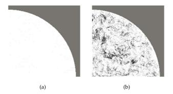
**Figure 7.13:** In-plane vectors, depicting the secondary flow structure (a) up- and (b) downstream of the foam sample for a Reynolds number of about  $\text{Re}\approx 6'000$ .
