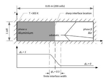
**Figure 6.2:** Outline of the one dimensional test case together with an indication for the profile of the order parameter  $\phi_{\alpha}$ . The sharp interface location corresponds to  $\phi_{\alpha} = \phi_{\beta} = 0.5$ .
