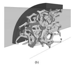
**Figure 7.3:** (a) Basic foam geometry (dimensions  $2.2 \text{ cm} \times 2.2 \text{ cm} \times 2.2 \text{ cm}$ ) imported in StarCCM (b) customised sample geometry reflecting the real sample geometry and flow situation.
