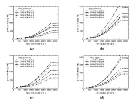
**Figure 3.15:** Pressure loss for all the individual foam samples of (a) 10 ppi aluminium, (b) 20 ppi aluminium, (c) 30 ppi aluminium and (d) 10 ppi copper, respectively. Reynolds number is based on inlet diameter.
