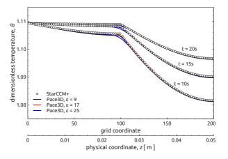
**Figure 6.13:** Interpolation of material properties k and  $C_V$ , interpolation of thermal diffusivity a and temperature profile, using decaying factorised inverse/harmonic interpolation in  $C_V$  for different diffuse interface widths,  $\epsilon$  and at different instances of time.
