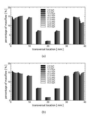
**Figure C.8:** Massflow distribution along transversal direction for 30 ppi aluminium foam of 100 mm length at (a) inlet and (b) outlet.
