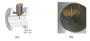
**Figure 3.9:** Detailed view on (a) the three dimensional design models of the custom made pressure probe section of the test rig (linear actuator and sensor are omitted here) and (b) image of the Pitot tube inside the 'real' assembly.
