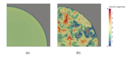
**Figure 7.11:** Distribution of velocity magnitude (a) up- and (b) downstream of the foam sample for a Reynolds number of about  $\text{Re}\approx6'000$ .
