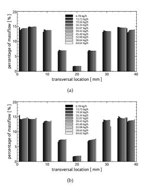
**Figure C.2:** Massflow distribution along transversal direction for 10 ppi aluminium foam of 100 mm length at (a) inlet and (b) outlet.
