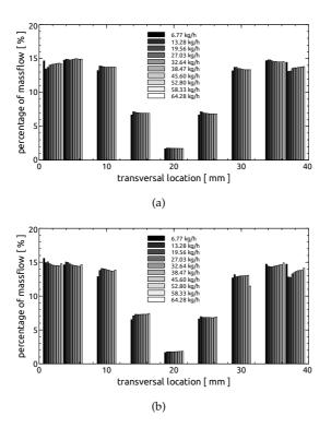
**Figure C.4:** Massflow distribution along transversal direction for 20 ppi aluminium foam of 100 mm length at (a) inlet and (b) outlet.
