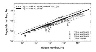
**Figure 3.19:** Correlation of the non-dimensional pressure loss per unit length and non-dimensional velocity, in terms of Hagen and Reynolds number for all foam types and lengths.
