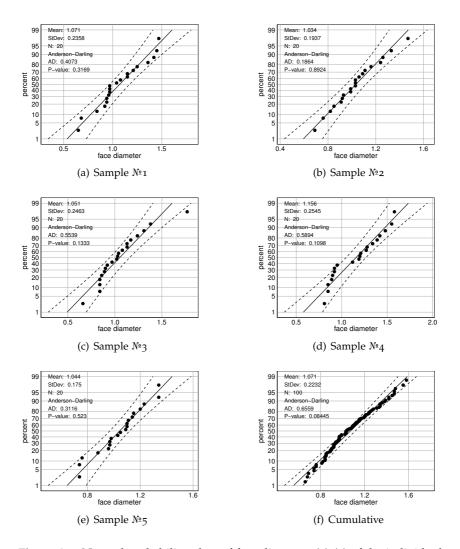
**Figure A.6:** Normal probability plots of face diameter, (a)-(e) of the individual 20 ppi aluminium samples 1-5 and (f) cumultative normal probability plot.
