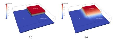
**Figure 8.1:** Exemplary application of the segmented tensorial mobility multiphase formulation. Heat conduction in a ternary 2D domain: (a) initial temperature distribution and (b) snapshot of the steady temperature distribution.
