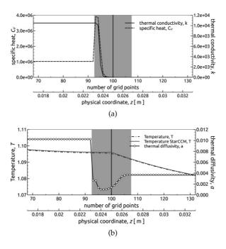
**Figure 6.10:** Inverse/harmonic interpolation in *k* and factorised inverse/harmonic interpolation of  $C_V$  using a single decaying factor. (a) interface profile  $\phi$  together with material properties *k* and  $C_V$ , (b) temperature profile, interface profile  $\phi$  and thermal diffusivity *a*. The shadowy area indicates the diffuse interface region, with a vertical line at  $\phi = 0.5$ .
