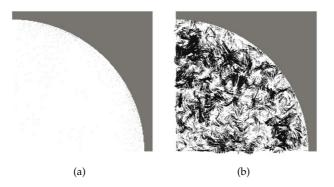
**Figure 7.14:** In-plane vectors, depicting the secondary flow structure (a) up- and (b) downstream of the foam sample for a Reynolds number of about  $\text{Re} \approx 26'000$ .
