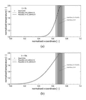
**Figure 6.23:** Temperature profiles across the concave interface (circular inclusion of air inside aluminium) for two different interface widths, 6 cells and 15 cells, respectively, after (a) two seconds and (b) ten seconds, each compared to the numerical reference solution obtained with StarCCM. The shadowy regions mark the diffuse interface layer.
