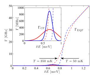
**Figure 2.** Transition rate as a function of energy difference for both equilibrium quasiparticles (dashed red/blue) and incoherent Cooper-pairs (solid red/blue), with  $E_j = E_c/20$ . The P(E) peak (centred around  $\delta E = 4E_c$ ) and the superconducting step edge of the quasiparticle transition are broadened as a function of temperature. Close to  $\delta E = 2\Delta$  we see that the rate of quasiparticle and Cooper-pair transitions occur at similar rates.
