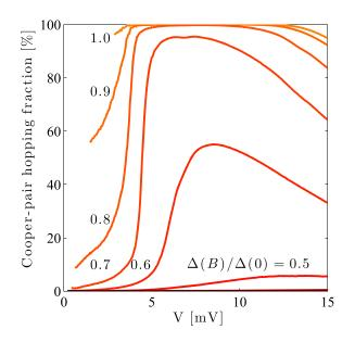
**Figure 8.** The relative fraction of Cooper-pair hopping as a percentage of the total hopping events within the array, as a function of both voltage and magnetic field (plotted for I > 0.5 aA). At zero magnetic field ( $\Delta(0) = 340 \,\mu eV$ ), the transport is almost entirely dominated by incoherent Cooper-pair hopping. As the magnetic field is increased ( $\Delta(B) \rightarrow 0$ ) the role of Cooper-pair hopping decreases and quasiparticles dominate.
