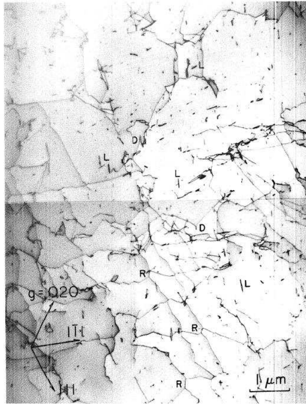
Figure 5.14.: Typical network structure of irregular shaped screw dislocations formed in Mo reproduced from [98]. R denote the junctions with Burgers vector of \langle 100 \rangle type. D and L denote the dipole trails and dipole loops respectively.
