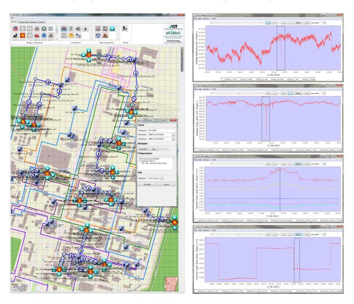
The model contains the available grid component specifications. The active power values based on the 10 minutes smart meter power consumption data at KIT-CN and the 5kHz sampled high rate EDR voltage data are used as input for the simulation model. GridLAB-D manages the data synchronization for the multi-rate input time series and performs the calculation of the power flow with
