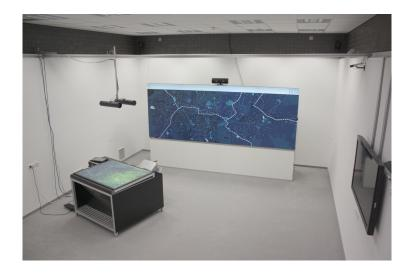
Figure 1.1: The Smart Control Room laboratory at the Fraunhofer IOSB in Karlsruhe, Germany: a research platform for multimodal, multi-user, multi-display interaction through computer vision and related technologies.
