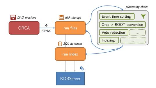
Figure 3.5: Flow diagram of the automated run processing chain. Once the DAQ machine has finished a data-taking run, the raw data is 'rsynced' to central file storage. The processing script performs various conversion / indexing steps and writes the converted data to the file storage and SQL databases, where it can be accessed by the service layer (KDBServer).
