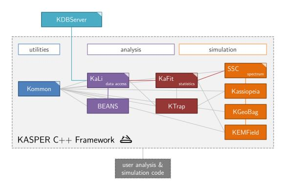
Figure 3.3: Schematic overview of KASPER's main components and their relation to each other. A brief explanation of each individual module is given the main text (section 3.2.1). Modules tagged with a white triangle were developed or significantly extended in the course of this thesis (Kommon, KaLi, KDBServer, SSC, KaFit).
