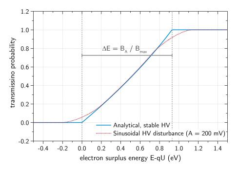
Figure 5.6: Transmission function for isotropically emitted electrons at a retarding energy of 18570 eV. The solid curve depicts the analytical form of T(E, 18570 eV), the dotted 'broadened' curve incorporates a sinusoidal high voltage fluctuation of the retarding potential.
