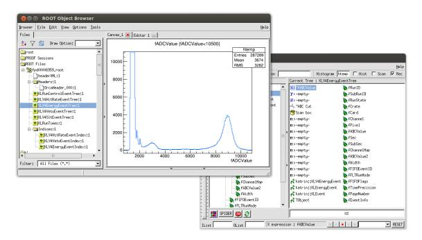
Figure 3.6: Structure of ORCA detector data in ROOT compatible format, opened with the TTreeViewer tool provided by ROOT. A histogram of energy ADC values can easily be obtained with only a handful of mouse clicks.
