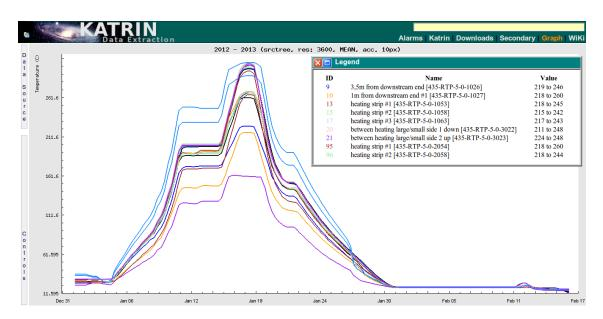
Figure 2.10: ADEI web frontend showing a graph of several temperature sensors (in °C) during the spectrometer bake-out in January 2013.
