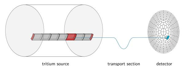
Figure 5.14: The source segmentation is performed dynamically along the beam direction,
