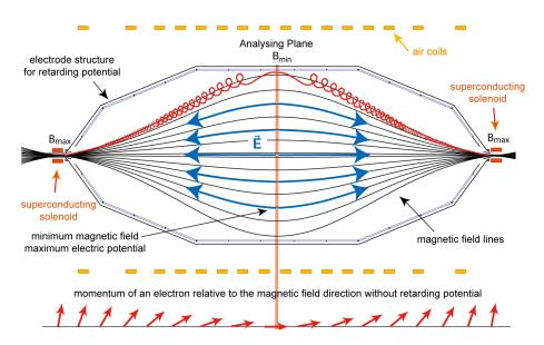
**Figure 2.3:** Working principle of a MAC-E filter. Electrons traveling on cyclotron paths along the guiding magnetic field lines undergo an adiabatic momentum transformation. The direction of their momentum vector is being parallelized along the field lines in regions of low magnetic field strength (analyzing plane), where the electrons can be precisely analyzed by the electrostatic retarding potential. Figure adapted from [Hug08].
