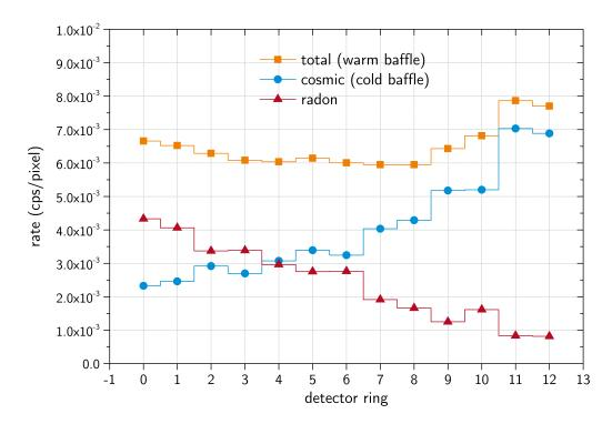
Figure 7.1: Background rates recorded during SDS-I commissioning and plotted for individual rings of the main detector. Index 0 = bullseye, 12 = outer ring.
