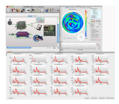
Figure 2.9: Screenshot of ORCA's graphical user interface, showing real time event monitoring of the focal-plane detector system.
