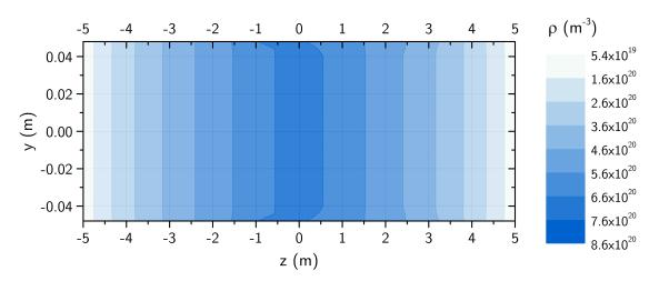
Figure 5.8: Gas density profile of the WGTS beam tube, calculated with SSC.
