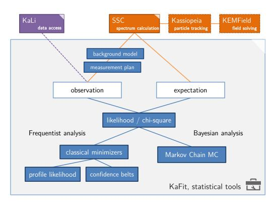
Figure 6.1: Schematic diagram of the components within KaFit, required for parameter inference and confidence interval construction.
