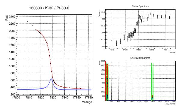
**Figure 4.8:** Monitor spectrometer filter spectrum (red line) and a fit of the K-32 conversion line (blue). Script written by Martin Slezák [Sle].
