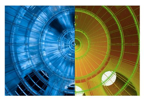
**Figure 2.4:** View into the main spectrometer along the beam axis facing towards the detector. The inner surface is covered with the two-layer wire electrode system. In this picture the three pump ports, visible at the bottom, are still empty. The left half shows a real photograph, while the right half depicts a discretized 3D model with the color indicating the electric potential calculated with the KATRIN field solving software KEMField. By courtesy of T.J. Corona [Cor14].
