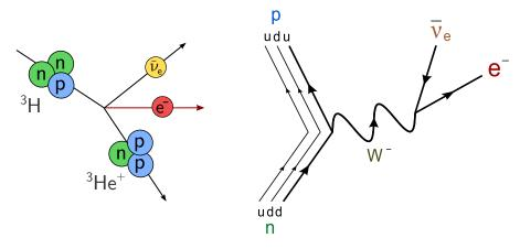
Figure 1.7: Schematic of the tritum  $\beta$ -decay.
