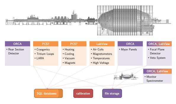
Figure 3.4: Illustration of various KATRIN data producers categorized by data acquisition system.
