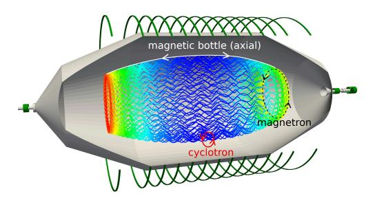
Figure 4.10: Track of a stored particle inside the main spectrometer, simulated with Kassiopeia and visualized with ParaView [Ced06]. Graphic by courtesy of Stefan Groh, KIT [Gro15].
