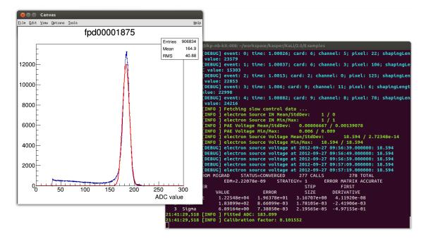
Figure 4.6: Energy calibration of the focal plane detector, purely built on KaLi analysis logic.
