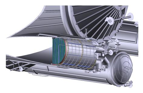
Figure 2.5: Cross section through one of the three main spectrometer pump ports, exposing the non-evaporable getter (NEG) pump and the liquid nitrogen cooled baffles (vertical blue blades on the left end of the pump port).
