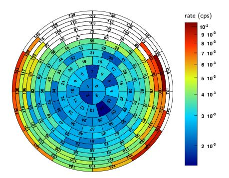
Figure 7.2: Pixel-view of accumulated detector events during a 12 h background measurement with active radon suppression (see main text). The total background rate amounts to 457 mcps. When correcting for the number of shadowed and non-active pixels (white), the rate normalizes to 614 mcps.
