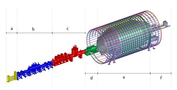
Figure 2.2: The KATRIN experimental setup, 70 m in length.
