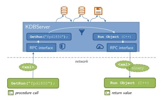
**Figure 3.10:** A client tool invokes a function, which is translated into a XML message. KDBServer parses the request, checks user permissions and assembles the data. The result is converted into an XML response (with binary attachments if necessary) and returned to the client.
