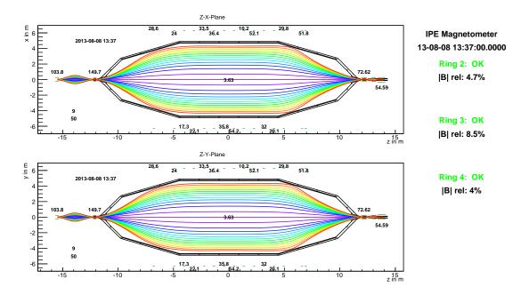
Figure 4.11: Near-time magnetic fieldline monitoring. The magnetic field calculation is based on real-time magnetometer data from 72 channels, accessed through the KaLi data interface.
