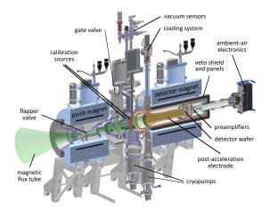
Figure 2.6: Focal plane detector setup.
