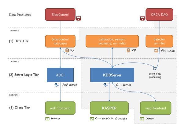
Figure 3.1: Diagram of the multi-tier IT infrastructure of the KATRIN experiment. A detailed explanation of the individual components is given in chapter 3 (tier 1 and 2) and chapter 4 (tier 3). Components within the shaded area were designed and in large parts implemented as part of this thesis.
