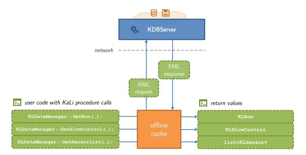
Figure 4.5: Data operations articulated to KLDataManager via function calls are accumulated into as little XML requests as possible. The returned data is intercepted by KaLi's caching mechanism and stored on the user's harddrive. When the request is repeated while a network connection us unavailable, KaLi will automatically attempt to fall back to cached data and return a result.
