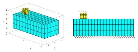
Figure 6.23: Initial configuration (left) and boundary conditions (right).
