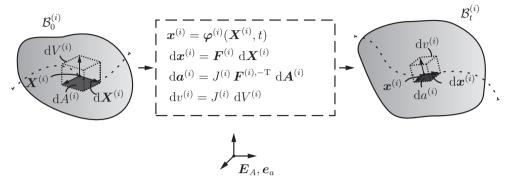
Figure 3.2: Relations between reference and current configuration for points, line-, areaand volume-elements.
