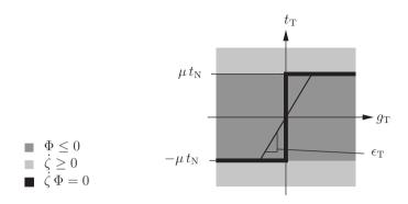
Figure 3.9: Admissible region for tangential traction  $t_{\rm T}$  with respect to the tangential gap  $g_{\rm T}$  in case of Coulomb law (one dimensional illustration, cf. Laursen [97]).
