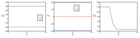
Figure 6.34: Linear (left), angular momentum (middle) and total energy (right) of the blocks with Coulomb coefficient of friction of  $\mu = 0.8$ .
