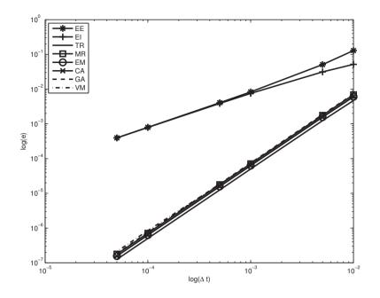
Figure 6.5: Error plot of different integrators for the soft spring with reference solution computed by the midpoint rule and a time step size of  $\Delta t = 10^{-6}$
