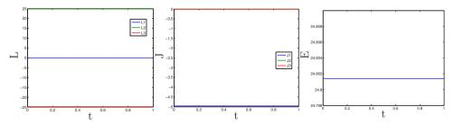
Figure 6.10: Linear (left), angular momentum (middle) and total energy (right) of the ball plate impact example corresponding to the EMS.
