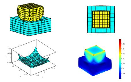
Figure 6.27: Deformed configuration (upper left) with top view (upper right), segmentation (lower left) and Von Mises stress (lower right) after the first translational movement (t = 1).
