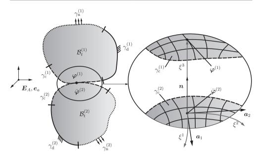
Figure 3.7: Parametrization of the spatial master surface  $\gamma_{\rm c}^{(2)}$ .
