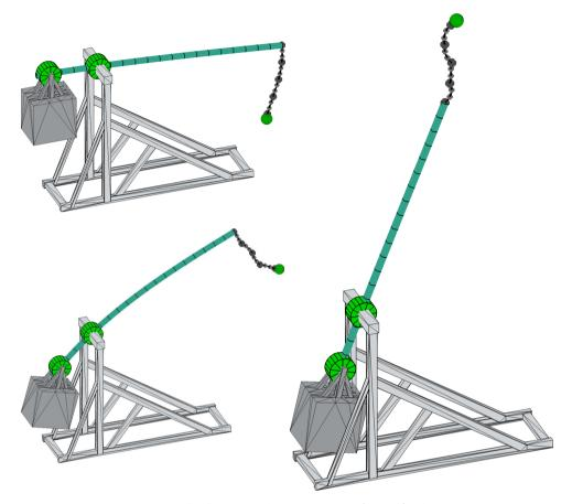
Figure 2.3: Trebuchet: Configuration after 50 time steps (top left), after 140 time steps (bottom left) and after 220 time steps (right).
