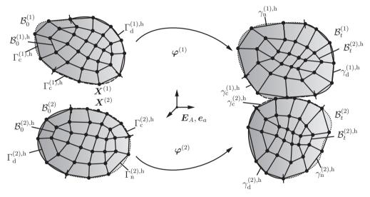
Figure 4.1: FE-discretization for the two-body contact problem.
