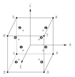
Figure C.1: Eight-point Gaussian quadrature rule for trilinear brick element.
