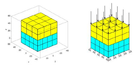
Figure 6.20: Initial configuration with loading and boundary conditions for the patch test.
