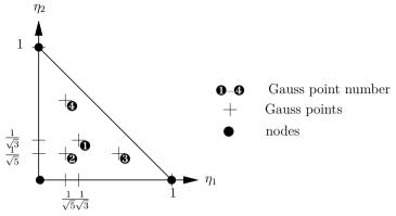
Figure 4.11: 4 point Gauss rule for triangular element.
