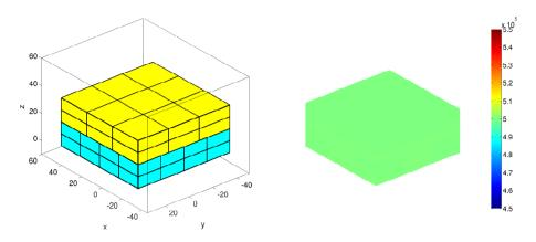
Figure 6.22: Displacement (left) and Von Mises stress distribution (right) of the patch test.
