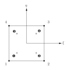
Figure C.2: Four-point Gaussian quadrature rule for trilinear brick element.
