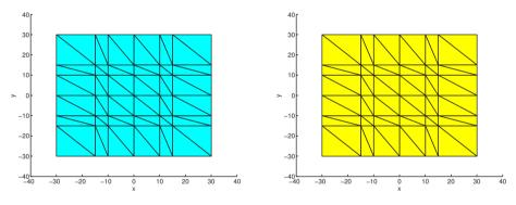
Figure 6.21: Initial segmentation of non-Mortar side (left) and Mortar side (right) for the patch test.
