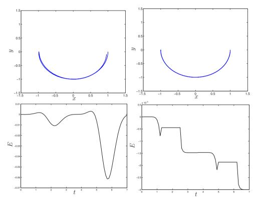
Figure C.4: Trajectory (upper) and energy (lower) plots of the ODE system (left) and of the reduced DAE system (right) using a time step size  $\Delta t = 0.1$ .
