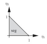
Figure 4.10: Triangular reference element of segment  $e_{\bar{s}}$ .
