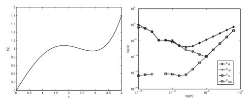
Figure D.1: Function f(x) (left) and error plot of numerical tangents ( $\varepsilon_{\rm fd}$ : forward finite difference,  $\varepsilon_{\rm bd}$ : backward finite difference,  $\varepsilon_{\rm cd}$ : central finite difference and  $\varepsilon_{\rm csd}$ : complex-step derivative) for function f(x) at x = 2.
