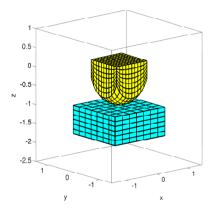
Figure 6.26: Initial configuration of the indenter and the block.
