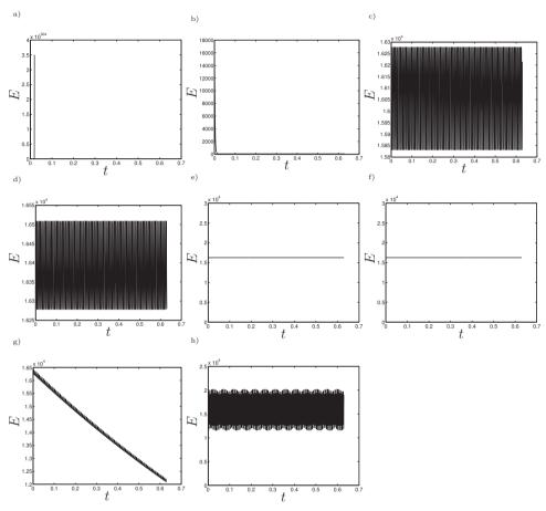
Figure 6.3: Energy plots for the stiff spring potential with time step size  $\Delta t = 5e$ -4: a) forward Euler method, b) backward Euler method, c) trapezoidal rule, d) midpoint rule, e) EMS, f) EMS based on CAT, g) generalized- $\alpha$  method  $(\rho = 0.7)$  and h) variational midpoint scheme  $(\alpha = \frac{1}{2})$ .
