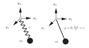
Figure 6.1: Spring (left) and string pendulum (right).
