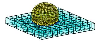
Figure 6.7: NTS projection at time t = 0.33 with slave nodes (yellow circle) and projected master nodes (blue x-mark).
