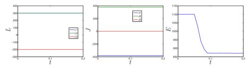
Figure 6.32: Linear (left), angular momentum (middle) and total energy (right) of the blocks with Coulomb coefficient of friction of  $\mu = 0.2$ .
