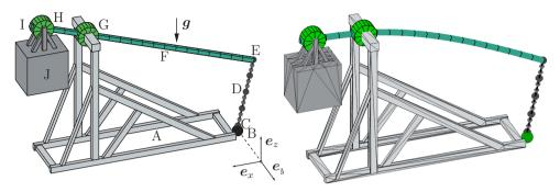
Figure 2.2: Trebuchet: Reference (left) and initial configuration with static equilibrium (right).
