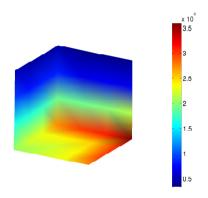
Figure 6.30: Initial Von Mises stress of the upper block with  $\mu = 0.8$ .
