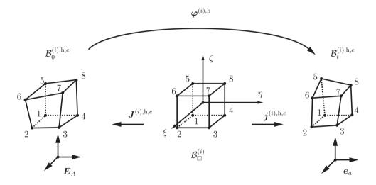
Figure 4.2: FE transformations on element level.
