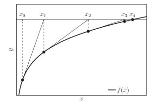
Figure A.1: Graphical illustration of the iteration process for Newton's method using the function  $f(x) = \ln(x) + \sqrt{x} - 2$ .
