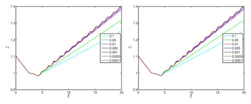
Figure 6.12: z-position of node 8 plotted over time (left: direct approach, right: augmented approach) employing the backward Euler scheme.
