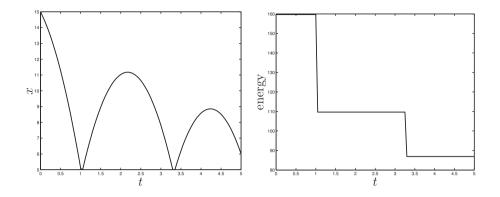
Figure 5.5: Active set strategy with standard constraint: configuration plot (left), energy plot (right).
