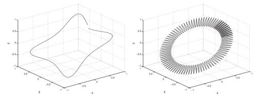
Figure 6.2: Reference (overkill) solution computed with midpoint rule ( $\Delta t = 1e$ -6) for soft ( $c = 10^3$ , left) and stiff ( $c = 10^6$ , right) spring potential (see Gonzalez and Simo [46]).
