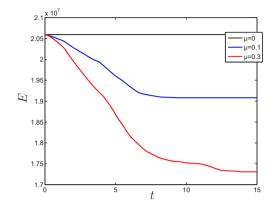
Figure 6.17: Total energy plotted over time (black line: frictionless EMS from Hesch and Betsch [61], colored lines: frictional CAT).
