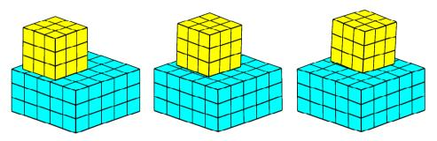
Figure 6.31: Snapshots of the blocks at t = 0.06 (left), t = 0.13 (middle) and t = 0.20 (right) with Coulomb coefficient of friction of  $\mu = 0.2$ .
