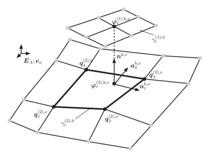
Figure 4.4: Five node NTS contact element with slave  $(\bullet)^{(1)}$  and corresponding master interface  $(\bullet)^{(2)}$ .
