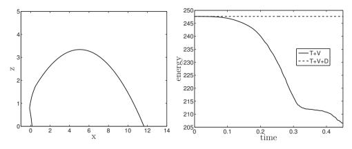
Figure 2.4: Trebuchet projectile: x-z trajectory (left) and energy plot (right).
