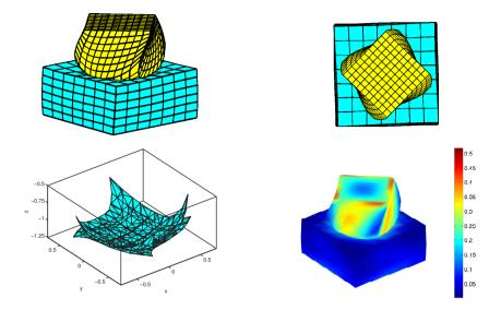
Figure 6.28: Deformed configuration (upper left) with top view (upper right), segmentation (lower left) and Von Mises stress (lower right) after the final rotational movement (t = 2).
