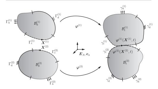
Figure 3.6: Configurations of the two body contact problem  $(\mathcal{B}_0^{(i)})$ : bodies in the reference configuration,  $\mathcal{B}_t^{(i)}$ : bodies in the current configuration).
