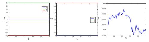
Figure 6.8: Linear (left), angular momentum (middle) and total energy (right) achieved for the ball plate impact example corresponding to the midpoint rule.
