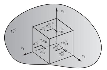
Figure 3.4: Components of the Cauchy stress tensor.
