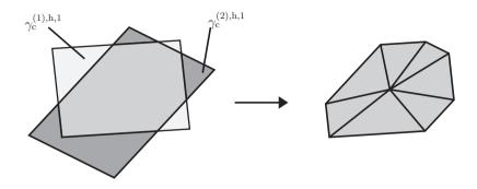
Figure 4.5: An overlapping Mortar and non-Mortar element (left), the identification as polygon and triangularization (right).
