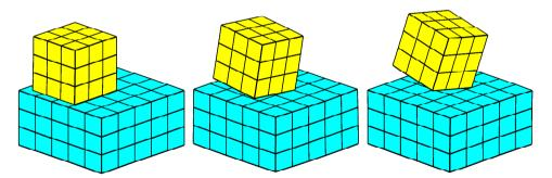
Figure 6.33: Snapshots of the blocks at t = 0.06 (left), t = 0.13 (middle) and t = 0.20 (right) with Coulomb coefficient of friction of  $\mu = 0.8$ .
