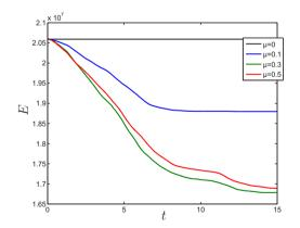
Figure 6.38: Total energy plotted over time (black line: frictionless EMS from Hesch and Betsch [62], colored lines: frictional Mortar approach).
