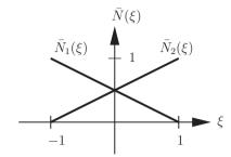
Figure 4.3: One dimensional linear local shape functions.
