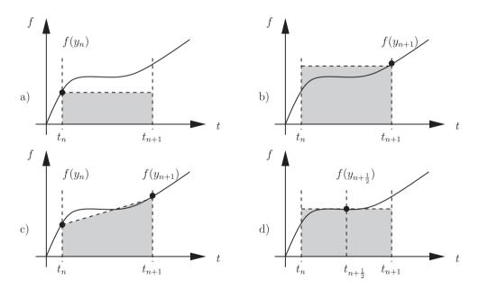
Figure 5.2: Integration of a typical 1D function  $f(y) : \mathbb{R} \to \mathbb{R}$  with a) forward Euler method, b) backward Euler method, c) trapezoidal rule and d) midpoint rule.
