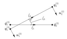
Figure 4.8: Intersections of the element edges of  $\partial \gamma_c^{(2),h,\bar{s}}$  and  $\partial \bar{\gamma}_c^{(2),h,\bar{s}}$  for an element couple  $\bar{s}$ .
