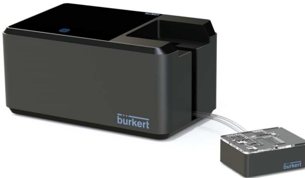
Figure 5.16.: Portable read-out device for the Lab-on-a-Chip system developed by Bürkert Fluid Control Systems. 111
