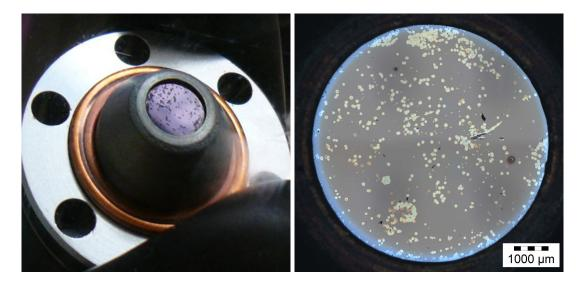
Figure 4.1.: Degradation of anti-reflection coated optical windows after contact with highly purified tritium gas. *Left:* Window in dismounted vacuum flange (CF16) with spot-like damaged areas on the tritium facing window side. *Right:* Microscopy image of the damaged AR coating of another window, acquired at Fusion Material Laboratory (IAM-WBM, KIT). Details in chapter 5.
