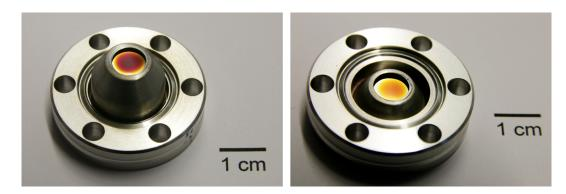
Figure 5.13.: Raman (left) and laser (right) window after magnetron sputtering. The coatings were illuminated under an obtuse angle to make the coating visible. The coatings do not fully reach to the edge of the windows due to the shadowing effect by the surrounding vacuum flange. This does not impose an issue for their functionality.
