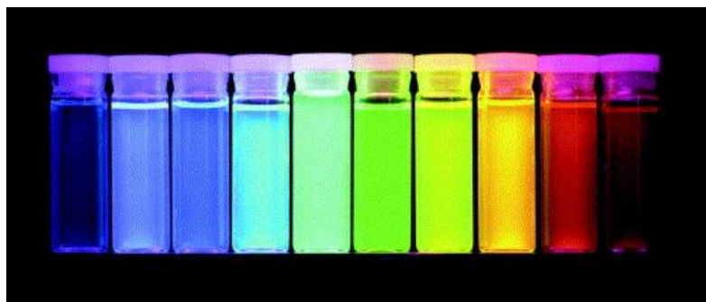
Figure 12. Ten distinguishable emission colors of ZnS-capped CdSe QDs excited with a near-UV lamp. From left to right (blue to red), the emission maxima are located at 443, 473, 481, 500, 518, 543, 565, 587, 610, and 655 nm. (Figure adapted from Ref. 202 with permission.) [202]
