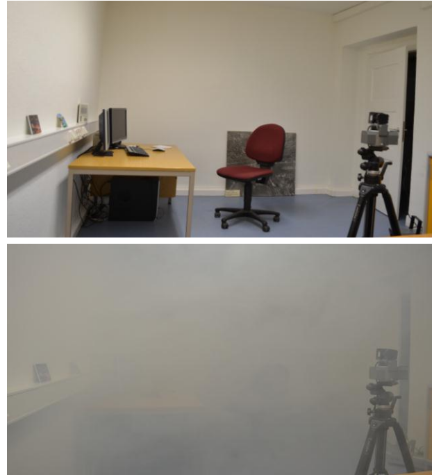
Figure 7: Example scene captured during the experiment; above: image captures one side of empty test office scene; below: the same scene under smoke.
