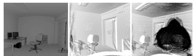
Figure 3: Overview of captured data: office room (left and middle: office without smoke, right: office with presence of smoke cloud).
