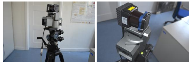
Figure 5: Laser scanner device with scanning unit.
