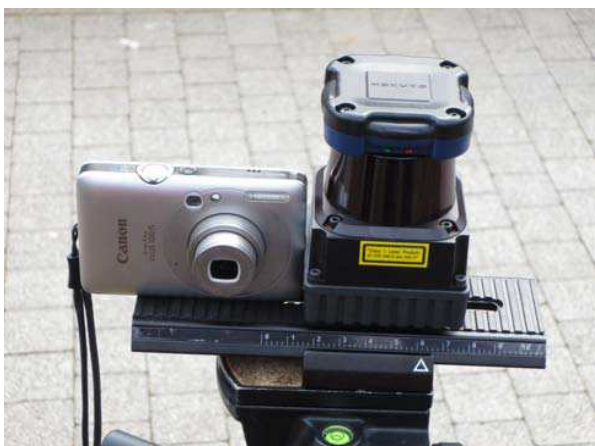
Figure 1. The two sensor devices utilized for the experiments: digital camera (Canon Digital IXUS 100 IS) and lightweight laserscanner (Hokuyo UTM-30LX-EW).
