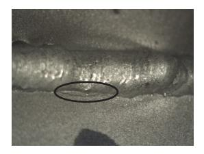
Figure 6: Crack adjacent to weld after assembly
