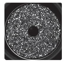
Fig. 4. CMT cut through beryllium pebble bed at z/d=0.5; d=1mm,  $D_0=49mm$ , Di=10mm.
