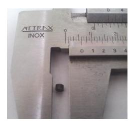
Fig. 6 Be-Ti sample for XRD investigations
