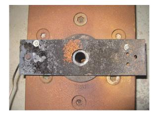
Fig. 3 (above). A copper plate as a beam current detection probe in front of the electromagnet core. The channel for the electron beam through an electromagnet pole is visible in the centre.
