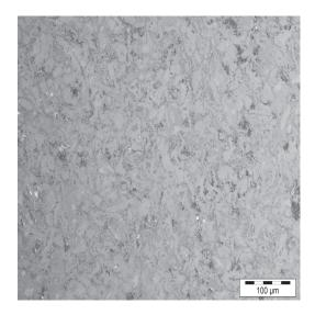
Fig. 5 Polished cross-section of Be-Ti rod in the transverse direction with the respect to an extrusion axis
