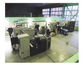
Fig. 3. Wire EDM machinig area for beryllium tiles manufacturing
