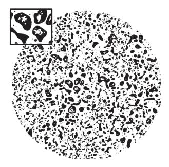
Figure 3: Same image as Fig.2 after application of the median filter and binarisation using the selected threshold. Artefacts within large pores may appear and should be removed.
