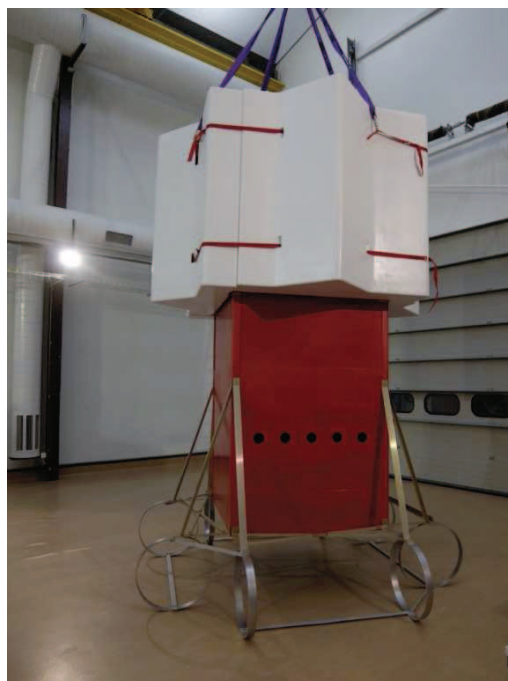
Figure 2.10: EUSO-Balloon gondola for balloon flight prepared for launch in Timmins, Ontario (Canada) [26].
