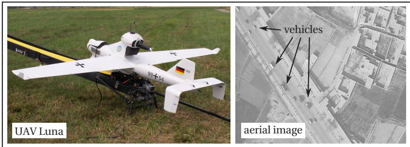
Figure 1.1: Luna UAV with a VIS camera and one example for an acquired aerial image.
