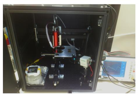
Figure 5.7.: Picture of the overall Kelvin Probe setup - It shows the black encasement and the experimental installations inside: The Kelvin probe head unit (red, central), the measurement platform with motorized stages (bottom center), the humidity stabilization system (bottom left) and the camera (bottom right).
