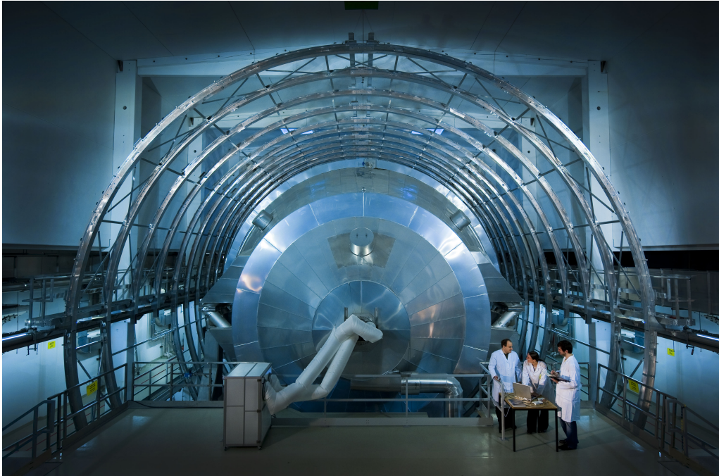
Figure 2.10: A photo of the main spectrometer from the pre-spectrometer side, with the latter not installed yet. The main spectrometer is 23.3 m long and has a diameter of 10 m. It is surrounded by a large air coil system. The picture was taken in 2009.
