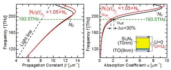
Figure 4.8 Dispersion relation of SPP guided by the Ag/ITO(8nm)/Si<sub>3</sub>N<sub>4</sub>(70nm)/Ag layer stack.Both, propagation constant and absorption coefficient, change when the carrier density of ITO is increased by 5 % (red lines). As opposed to the propagation constant the absorption coefficient varies significantly with ITO carrier density.
