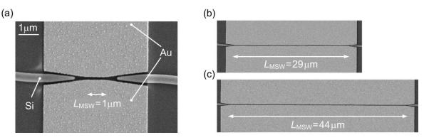
Figure 3.9 Fabricated metallic tapered mode converters with three different MSW lengths  $L_{\text{MSW}}$  of (a) 1 µm, (b) 29 µm, and (c) 44 µm. The slot size *h* is about 140 nm for all three devices.
