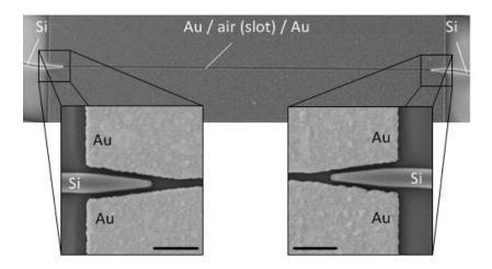
Figure 5.3 Scanning electron microscope image of the fabricated plasmonic phase modulator. The photograph is taken before coating with an electro-optic material. Black bars are one micrometer.
