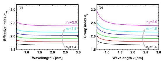
Figure 2.8 Effective and group refractive indices for an Ag-SiO2-Ag slab waveguide with a 100 nm thick SiO2 layer. (a) Effective refractive index and (b) group refractive index as a function of the operating wavelength for various insulator refractive indices from 1.4 to 2.0.
