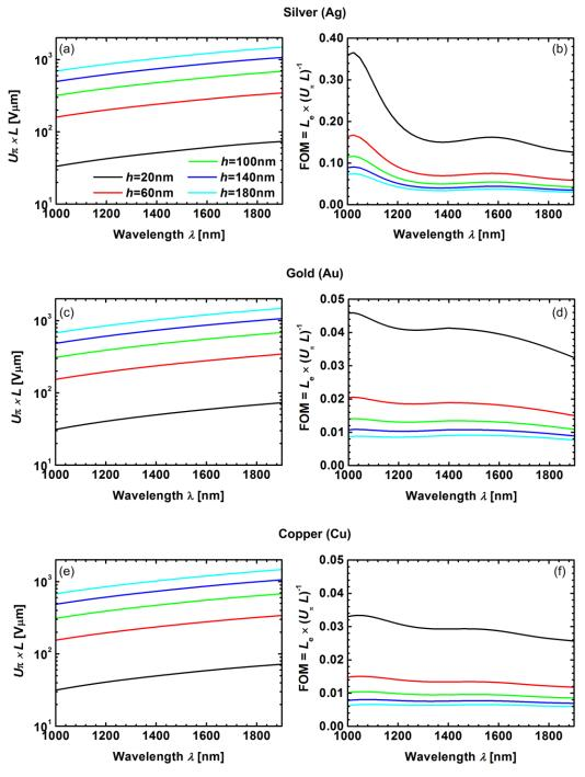
Figure 2.14 Characteristics of plasmonic phase modulators (PPMs) utilizing an electro-optic material with  $r_{33} = 70 \text{ pm} / \text{V}$ . The  $U_{\pi} \times L$  product and the FOM =  $L_e / (U_{\pi}L)$  are given for PPMs made of silver (a), gold (b) and copper (c) electrodes. The best device performance can be achieved in a PPM made of silver.
