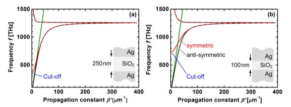
Figure 2.6 Dispersion relation of silver (Ag)-silicon dioxide (SiO2) -silver (Ag) MIM waveguide. Dispersion relation of both symmetric and anti-symmetric SPPs for an insulator thicknesses of 250 nm (a) and 100nm (b). The dispersion relation of a plane wave propagating in SiO2 is given as a green solid line.
