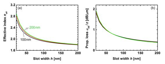
Figure 2.12 (a) Effective refractive index  $n_{\rm eff}$  and (b) power loss  $\alpha_{\rm dB}$  of a gap SPP at a wavelength of 1550 nm as function of slot width *h*. The results are given for three different metal thicknesses of 100 nm (black), 150 nm (red), and 200 nm (green).
