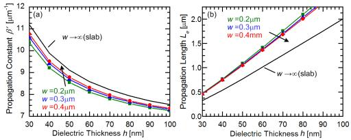
Figure 4.11 Influence of plasmonic 3D waveguide width w on propagation constant (a) and propagation length (b). For comparison, the 2D results from solving Eq. (4.4) are added (black line).
