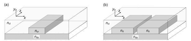
Figure 2.2 Examples of optical waveguide geometries. (a) Strip waveguide comprising a high refractive index  $n_{cr}$  core surrounded by a low index substrate and cladding materials with refractive indices of  $n_{sb}$  and  $n_{cl}$ , respectively. Light is guided along the *z*-axis confined in a core material due to the total internal reflection. (b) Slot waveguide comprising two rails with refractive indices  $n_{rl}$ . Light is confined to the low-index region of the slot between the rails.
