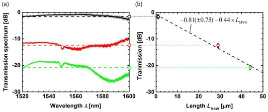
Figure 3.10 Measured transmission spectra of the fabricated MTMCs. (a) Transmission spectra for MTMCs with MSW lengths  $L_{MSW}$  of 1 µm (black), 29 µm (red) and 44 µm (green). Oscillatory features in the spectra are attributed to Fabry-Perot reflections in the device. (b) Power transmission versus device length  $L_{MSW}$ . Transmission spectra where the oscillations have been averaged on a linear scale are taken for estimation of the coupling loss.
