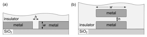
Figure 3.1 Metallic slot waveguides in two different configurations. (a) Vertically oriented and (b) horizontally oriented metallic slot waveguides.
