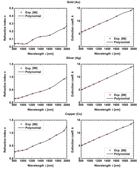
Figure 5.2 Measured and fitted complex refractive indices of silver, gold and copper.Red dots represent the measured refractive indices [86], while the black solid lines are the fitted curves with the polynomial of  $8^{\text{th}}$  order.
