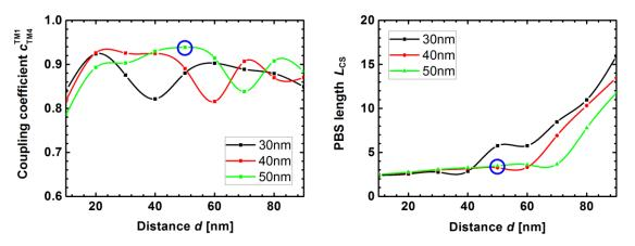
Figure 3.13 (a) Coupling efficiency of the quasi-TM mode at Port 1 to the quasi-TM mode at Port 4 and (b) the corresponding coupling length  $L_{CS}$ . The quasi-TM mode at Port 1 can be efficiently coupled to Port 4 in a PBS with a sub-5  $\mu$ m length. Geometrical properties taken within the blue circles are considered in the operating bandwidth study by performing finite integral technique simulations.
