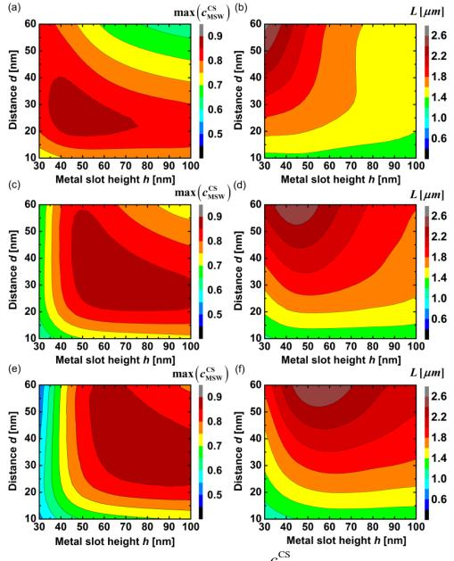
Figure 3.4 (a), (c), (e) Conversion efficiency  $C_{MSW}^{\infty}$  and (b), (d), (f) optimum CS length L for a MSW with a width w of 200 nm and for various cladding materials: (a) and (b) for glass, (c) and (d) for organic materials with refractive indices of 1.6, and (e) and (f) for refractive index of 1.7.
