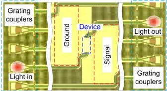
Figure 5.5 Optical microscope image of the modulator fabricated on the SOI platform.Light is launched into the silicon nanowire using standard diffraction grating couplers. The photonic mode polarized parallel to the substrate is guided to the device. The photonic-plasmonic mode conversion is accomplished by a metal taper coupler. The SPP is then guided through the modulator and converted back to the photonic mode. Light is detected at the output diffraction grating.
