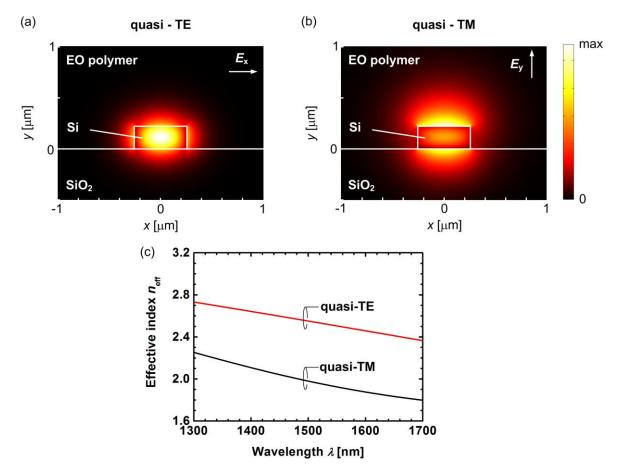
Figure 2.3 Fundamental quasi-TE and quasi-TM modes of a silicon strip waveguide with an EO organic cladding.(a) Field profiles of a quasi-TE (a) and a quasi-TM (b) modes and corresponding effective refractive indices (c).
