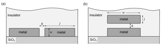
Figure 2.9 Cross-sections of 3D metallic slot waveguides (MSW) with (a) vertically orientated (vertical MSW) and (b) horizontally oriented slots (horizontal MSW).
