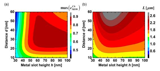
Figure 3.5 Conversion efficiency and coupling length for a horizontal MSW with a width w of 300 nm and a cladding refractive index of 1.7. (a) Conversion efficiency and (b) coupling length for various distances d and slot sizes h.
