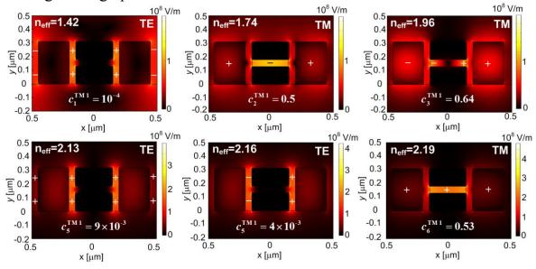
Figure 3.12 Supermodes of the polarization beam splitter (PBS) with d = 50 nm and h = 50 nm. The amplitude coupling efficiency  $c_{\mu}^{\text{TMI}}$  for quasi-TM excitation at Port 1 is given below each mode profile. The relative phase of the dominating electric field component in the cross-section ( $E_y$  or  $E_x$  for quasi-TE or quasi-TM, respectively) is represented with (+) and (-)-signs. Second, third and sixth supermode when excited by a quasi-TM at port 1 (left-hand side SWG).
