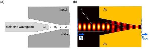
Figure 3.7 Metallic tapered mode converter (MTMC) that can be used to convert a dielectric waveguide mode in a gap SPP of a MSW. (a) Top view of a MTMC with a tapering angle of  $\theta$ , metallic slot width of h. (b) Electric field distribution in a MTMC between silicon strip waveguide with a width of and plasmonic metallic slot waveguides for a slot width of 140 nm and silicon strip.
