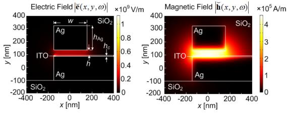
Figure 4.10 SPP mode profile in terms of dominating magnetic and electric field components at the active part of the modulator: Ag/SiO<sub>2</sub>(40nm)/ITO(8nm)/Ag.The fields are normalized to a cross-section power of 1 W. Similar to the slab structure,  $h_c$  and h define the ITO and dielectric thicknesses, respectively. In addition,  $h_{Ag}$  and W describe the thickness and the width of the top silver electrode.
