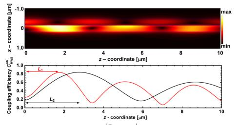
Figure 3.3 Electrical field distribution  $|\mathbf{\breve{E}}_{CS}(\mathbf{r},\omega)|_{y}$  in the mode converter with a width w of 300 nm, slot height of h of 60 nm is given for an organic cladding with a refractive index of 1.7. The conversion efficiency is given as a function of a length L for two different distances d of 20 nm (red) and 60 nm (black).
