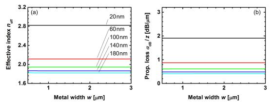
Figure 2.13 (a) Effective refractive index and (b) attenuation constant  $\alpha_{dB}$  of the gap SPP as a function of the metal width *l* for five different slot sizes of 20 nm (black), 60 nm (red), 100 nm (green), 140 nm (blue) and 140 nm (cyan).
