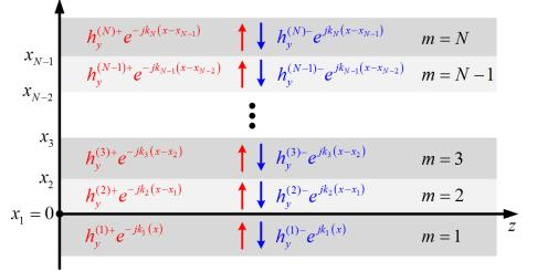
Figure 5.1 Multilayer slab waveguide.Layers m = 1 and m = N extend to minus and plus infinity, respectively. Layers m = 2...(N-1) have a finite thicknesses of  $x_m - x_{m-1}$ .
