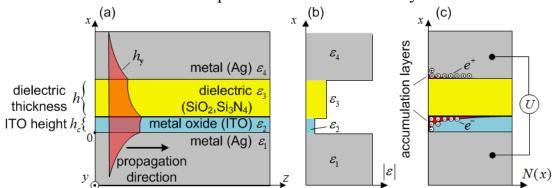
Figure 4.7 Plasmonic structure with metal/dielectric/metal-oxide/metal layers.(a) Geometry and (b) dielectric permittivity distribution. The  $h_y$  component of the SPP magnetic field is schematically shown as a contour filled with reddish color in (a). The SPP propagates along the positive z-direction. (c) Carrier density distributions N(x) in both electrodes
