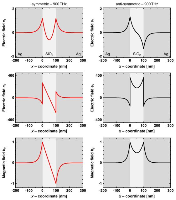
Figure 2.7 Symmetric and anti-symmetric SPPs of  $Ag-SiO_2$ -Ag waveguide with a  $SiO_2$  thickness of 100 nm. Non-zero components of the electric and magnetic transverse fields (middle and lower row) are plotted for the symmetric SPP (red solid line, left column) and for the anti-symmetric SPP (right column, black solid line). The upper row shows the longitudinal symmetric and anti-symmetric electric fields.
