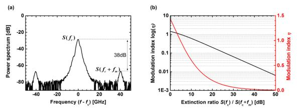
Figure 5.6 Spectrum of the sinusoidal phase modulated signal and its relation to the modulation index.(a) Optical spectrum measured after the1stG plasmonic phase modulator driven with an RF power of 8 dBm is given as an example of the spectrum of the sinusoidal phase modulated signal. (b) Modulation index is given as a function of the power ratio between carrier frequency and the first side band  $S(f_c)/S(f_c+f_m)$  carrier and first side.
