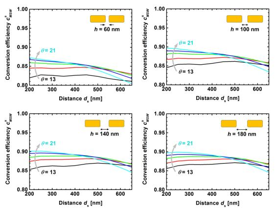
Figure 3.8 Amplitude conversion efficiency of a MTMC as a function of the distance  $d_s$  for five different taper angles  $\theta = 13^{\circ}(\text{black})$ ,  $15^{\circ}(\text{red})$  up to  $21^{\circ}(\text{cyan})$ . The amplitude conversion efficiencies are given for vertical MWSs with a slot width *h* of 60 nm (a), 100 nm (b), 140 nm (c) and 180 nm (d).
