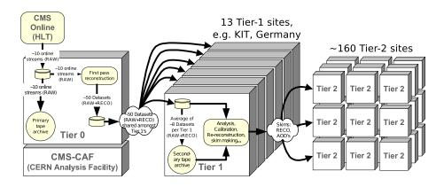
Figure 2.8.: Architecture of the CMS computing grid, taken from [71] with modifications. The RAW data format is stored at the Tier-0 sites at CERN and the Wigner research center for physics in Budapest. The 13 Tier-1 to date have large storage capacities and are responsible for save-keeping the RAW and RECO datasets. At the numerous Tier-2 sites and Tier-3 centers the AOD datasets for the analyses are saved.
