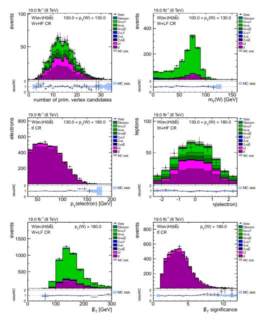
Figure 5.12.: Different event distributions in control regions for the W( $e\nu$ )H channel. Data/MC comparisons are shown for the low  $p_{\rm T}$  region (top row), intermediate  $p_{\rm T}$  region (middle row) and the high  $p_{\rm T}$  region (bottom row) in all three control regions as indicated in the figures. The number of events in simulation is normalized to data. The corresponding distributions for the W( $\mu\nu$ )H channel are presented in Figure A.1 in the appendix.
