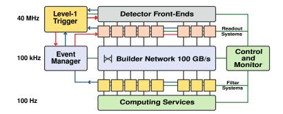
Figure 2.7.: Architecture of the CMS trigger and data acquisition system, taken from [71]. The two stages applied for event rate reduction from 40 MHz to 100 Hz are depicted. First, only events passing the hardware-driven Level-1 trigger requirements are forwarded to the readout systems. For these events the event builder combines the available detector information. In the end, the software-driven HLT filter system decides whether an event is stored or not.
